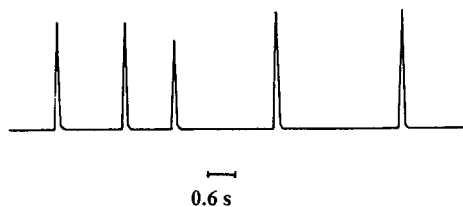
Fig. 2. Pulses of power being supplied to the heater of a modern chromatograph when operated at a relatively low temperature (40°C).
