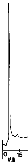
Fig. 5. Electropherogram of rabbit-anti-mouse antibodies, the major peak being IgG. Electrophoretic conditions: 5 mg/ml F-108 modified capillary, 43 cm length (31 cm effective length) \times 50 \mu m I.D.; 0.01 M phosphate buffer, pH 3.0; voltage: 15 kV; wavelength: 200 nm.
