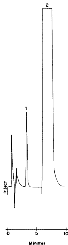
Fig. 1. Separation of nitrate in digested sample. Peaks: 1 = \text{NO}_3^- (0.88 mg/l); 2 = \text{SO}_4^{2-} .
