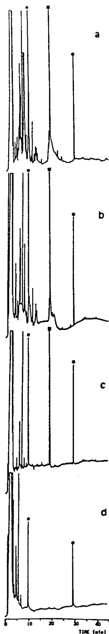
Fig. 2. (a) Chromatograms for a human milk sample, obtained by GC-ECD, (a) without any chemical treatment and after (b) acid, (c) alkali and (d) oxidant treatment. ★ = Peak at the same retention time as HCB; ◻ = peak at the same retention time as p,p' -DDE; ● = peak at the same retention time as methoxychlor. See text for operating conditions.
