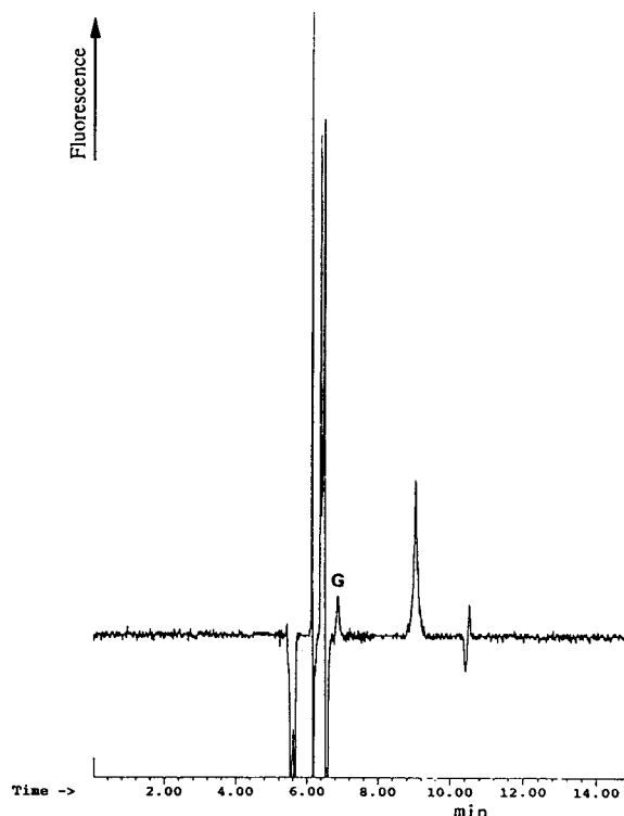
Fig. 5. Column-switching LC–FD of a surface water sample spiked with glufosinate at the 0.25 \mu\text{g/l} level. Chromatogram obtained after blank subtraction. LC conditions as in Fig. 4.
