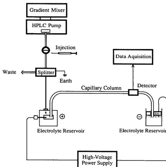
Fig. 1. Schematic representation of an electrochromatographic system.
