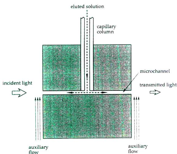
Fig. 1. Schematic of the post-column microchannel flow cell.
