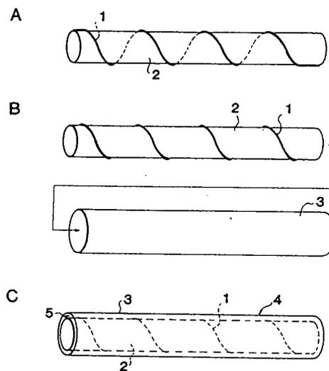
Fig. 1. Steps illustrating the construction of the concentric column. (A) Prepare a clad-removed fused-silica tube, used as the inner tube of the column, and wind a line helically around it; (B) insert the inner tube into a wider I.D. fused-silica tube; (C) completed. 1 = line; 2 = inner tube; 3 = outer tube; 4 = polyimide clad of outer tube; 5 = separation chamber.
