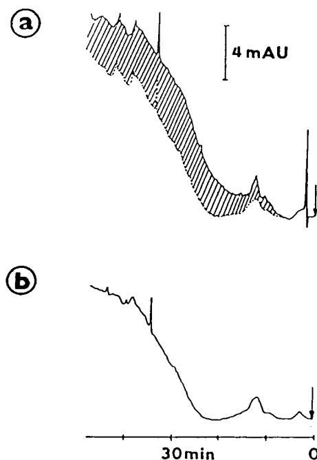
Fig. 9. HPLC profile of a humic acid sample at a detection wavelength of 240 nm. (a) 20- \mu l volume of the sample contained the acids at a 0.5 g/l concentration; (b) blank run under the same elution conditions (Table 1) as in (a). The shaded area in (a) indicates the shift of the detection signal on injection of the sample.
