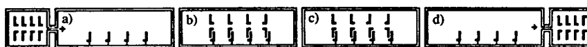
Fig. 3. On-column deracemization experiment. (a) racemate pumped onto column. (b) selective adsorption of one enantiomer leaves an excess of the opposite enantiomer in the mobile phase. (c) racemization of the analyte in the mobile phase. (d) column flushed to afford sample enriched in more retained enantiomer.
