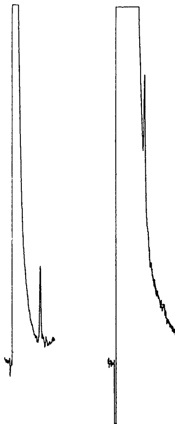
Fig. 2. RFD response of a trace sulfur peak on and off the solvent tail. The amount of injected analyte (1 ng thianaphthene) is precisely the same; however, the amount of solvent (acetone) has been increased 12 times for the second chromatogram by drawing additional acetone into the syringe prior to injection. The enhanced dip preceding the second solvent peak is due to the increased pressure surge caused by the sudden evaporation of a larger amount of acetone.
