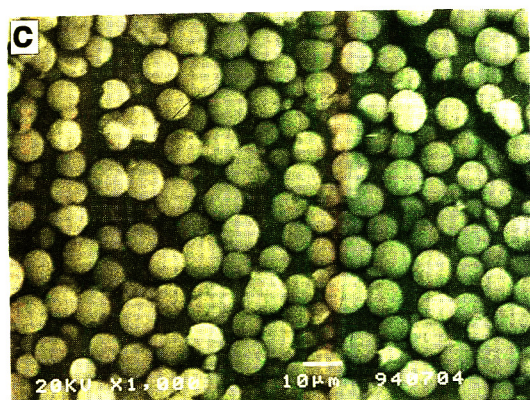
Fig. 3. Scanning electron micrographs of matrix silica and magnesia-coated silicas: (a) untreated silica; (b) 5400 ppm magnesia-coated silica dried at 110°C; (c) 5400 ppm magnesia-coated silica calcined at 800°C.
