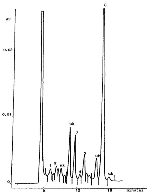
Fig. 7. High-performance liquid chromatogram. Sample solution of molasses 2%. Peaks: 1 = citric; 2 = malic; 3 = lactic; 4 = formic; 5 = acetic; 6 = pyroglutamic; uk = unknown.
