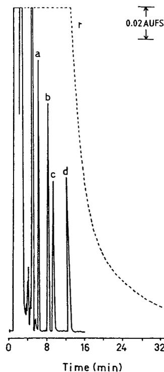
Fig. 3. Composite liquid chromatogram of 4-chlorophenol (MCP) (15 nmol), 2,4-dichlorophenol (DCP) (10 nmol) and 2,4,6-trichlorophenol (TCP) (10 nmol) derivatized with PEDAES with acid treatment (solid line) and without acid treatment (dashed line) after derivatization. Peaks: a = derivative of MCP; b = derivative of DCP; c = diphenyl (I.S.); d = derivative of TCP; r = excess of reagent. See text for conditions.
