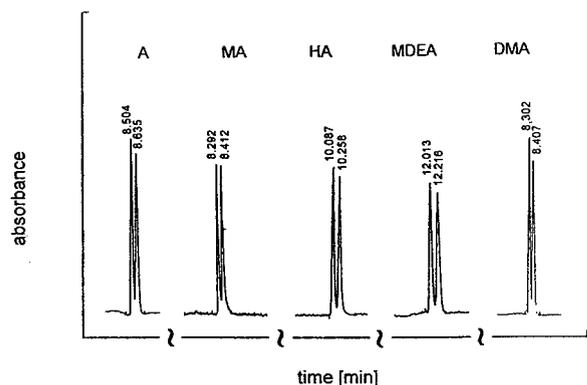
Fig. 2. Electropherograms of five well separated amphetamines using native  $\beta$ -CD as selector. Abbreviations as in Fig. 1. Experimental conditions: Non-coated fused-silica capillary with 50  $\mu$ m I.D., total length of 48.5 cm and effective length of 40 cm. Detection wavelength, 214 nm. BGE: aqueous solution of 50 mM sodium dihydrogenphosphate at pH 2.5, 10 mM  $\beta$ -CD; temperature, 20°C, applied voltage, 20 kV.
