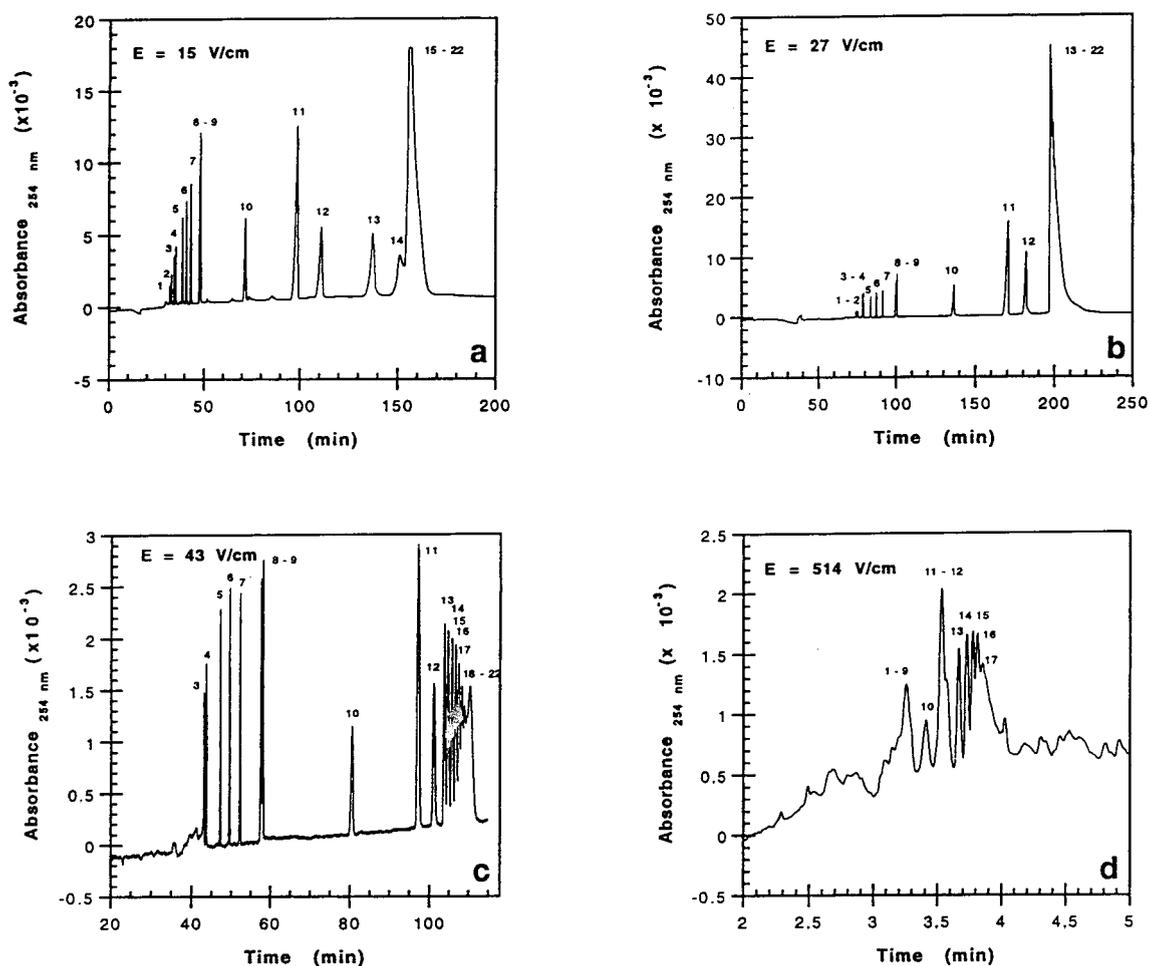
Fig. 3. Capillary electrophoresis of 1-kbp ladder under different electric field strengths, but at same polymer concentration (0.4% HPC), in 89 mM Tris–89 mM boric acid–2.5 mM EDTA–10  $\mu$ M ethidium bromide. Conditions and peaks as in Fig. 2.
