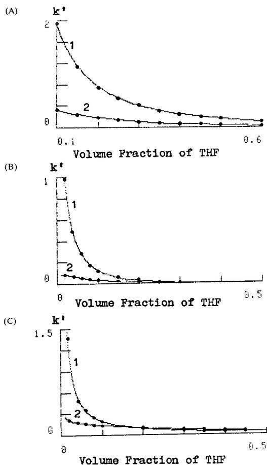
Fig. 1. Change in capacity factors of 4-nitrobenzoic acid (1) and 4-nitrobenzoyl chloride (2) with variation of the volume fraction of THF in eluent of the three Shim-Pack CLC columns: (a) C<sub>3</sub>; (b) C<sub>8</sub>; (c) C<sub>18</sub>.
