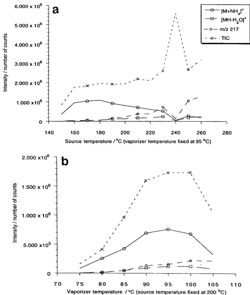
Fig. 4. Influence of (a) ion source temperature and (b) vaporizer temperature on the adduct molecular and fragment ions of armillyl orsellinate.
