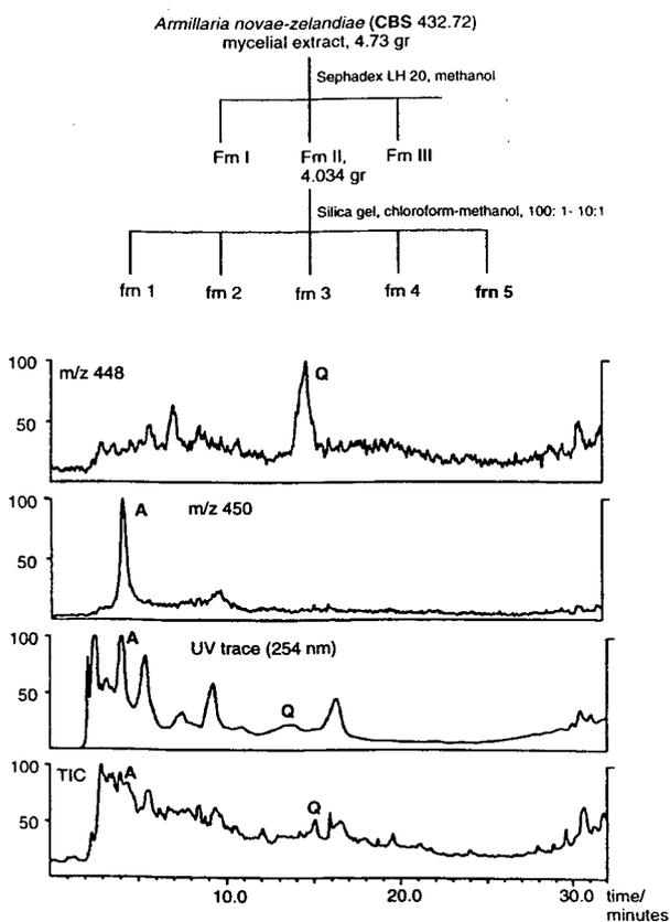
Fig. 8. LC–TSP–MS analysis of subfraction 5 of chromatographic separation of mycelial extract of *A. novae-zelandiae* (strain CBS 432.72) (see inset). The UV trace at 254 nm and TIC trace are displayed, in addition to selected-ion traces corresponding to adduct ions of 13-hydroxy-4-methoxymelleolide (D) and mellelidal (A).
