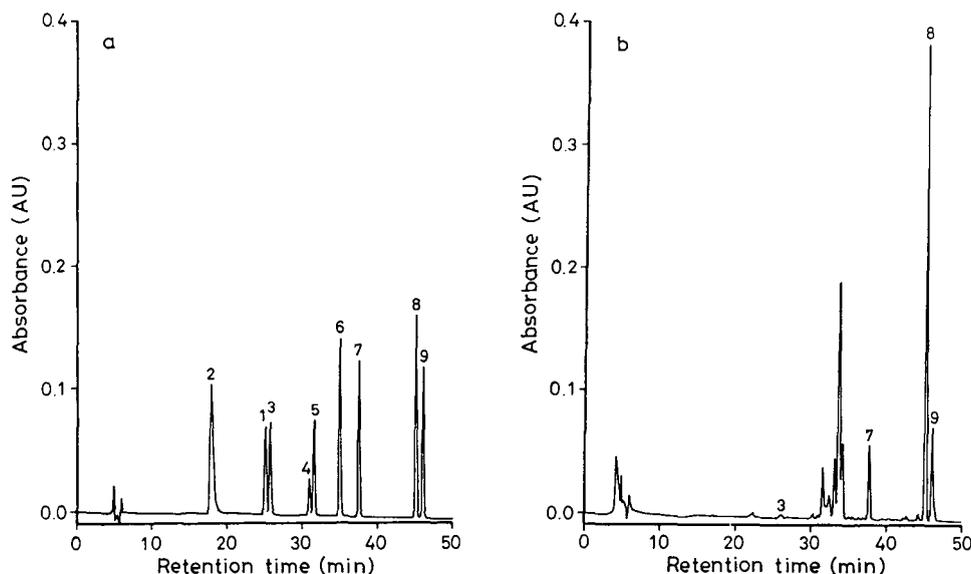
Fig. 2. HPLC of (a) a mixture of nine authentic coumarins and (b) an extract of *Angelicae Tuhou Radix*. Column: Cosmosil 5C<sub>18</sub>-AR (250 mm × 4.6 mm I.D., particle size 5 μm). Eluents: solvent A, H<sub>2</sub>O–CH<sub>3</sub>CN (8:2); solvent B, H<sub>2</sub>O–CH<sub>3</sub>CN–CH<sub>3</sub>OH (2:9:9). Elution profile: 0–40 min, 100–0% A (0–100% B); 40–50 min, 100% B. Detection: UV at 322 nm. Peak numbers as in Fig. 1.
