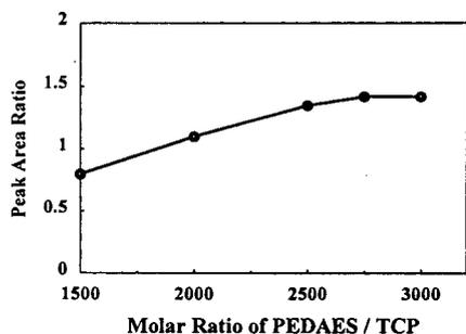
Fig. 2. Effect of molar ratio of PEDAES to 2,4,6-trichlorophenol on the formation of the TCP derivative. See text for conditions.
