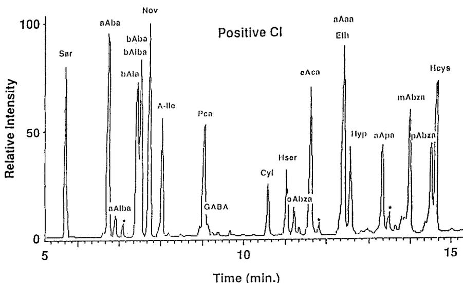
Fig. 1. Reconstructed TIC of positive chemical ionization GC-MS of the trifluoroethanol ECF derivatized non-protein amino acids. Peaks marked with an asterisk were not identified.
