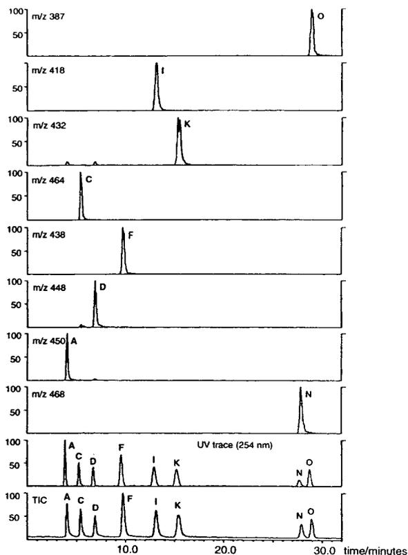
Fig. 5. LC-TSP-MS analysis for eight sesquiterpene aryl esters. For conditions, see Experimental. The UV trace at 254 nm and TIC trace for the standard solution are displayed, in addition to selected-ion traces corresponding to the adduct molecular ions of O, I, K, C, F, D, A and N.
