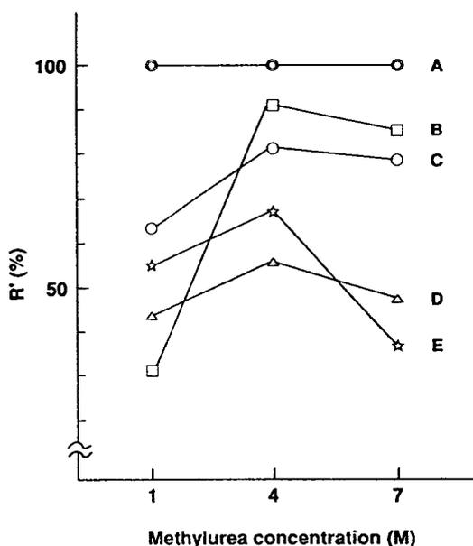
Fig. 2. Effect of methylurea concentration on enantioselectivity of  $\beta$ -CD (10 mM). Solutes: A = dansyl-D,L-aspartic acid, B = dansyl-D,L-leucine, C = dansyl-D,L- $\alpha$ -amino-*n*-butyric acid, D = dansyl-D,L-norleucine, E = dansyl-D,L-phenylalanine.
