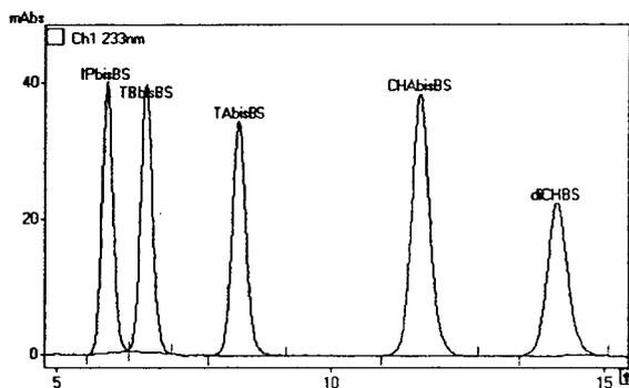
Fig. 2. Chromatogram of alkylbis(2-benzothiazolylsulfen)amides with N-dicyclohexyl-2-benzothiazolesulfenamide as internal standard using acetonitrile–methanol–water (7:1.5:1.5, v/v) as mobile phase at the flow-rate of 1.4 cm<sup>3</sup> min<sup>-1</sup> and  $\lambda_{\max}$  233 nm.
