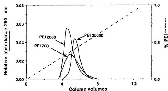
Fig. 3. LDH elution profile using a gradient of PEI. Experimental conditions:  $1.5 \times 1.0$  cm I.D. Red Sepharose column. A  $520\text{-}\mu\text{l}$  volume of pure LDH (1.1 mg/ml) was applied and eluted using a 0 to 1% linear PEI gradient at a flow-rate of 0.5 ml/min. The elution profiles are adjusted subtracting the contribution of PEI absorbance at 280 nm. Arrows indicate the molecular mass of PEI used.
