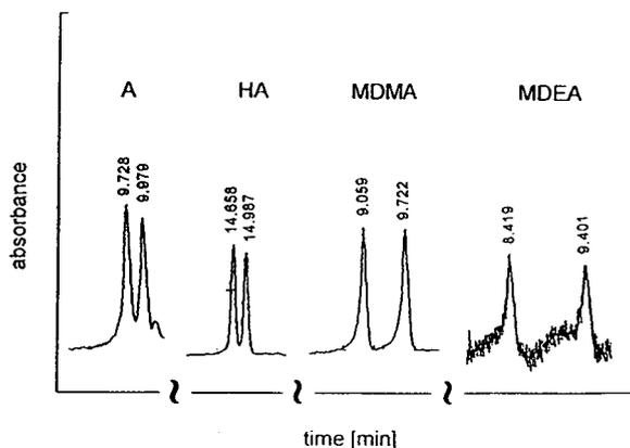
Fig. 4. Electropherograms of selected Marfey's reagent derivatized amphetamines applying nonchiral SDS micelles. Experimental conditions: Non-coated fused-silica capillary with 50  $\mu$ m I.D., total length of 48.5 cm and effective length of 40 cm. Detection wavelength, 340 nm. BGE: 80% (v/v) aqueous solution of 5 mM sodium borate at pH 9.0, 100 mM SDS, 20% (v/v) methanol; temperature, 40°C; applied voltage, 30 kV.
