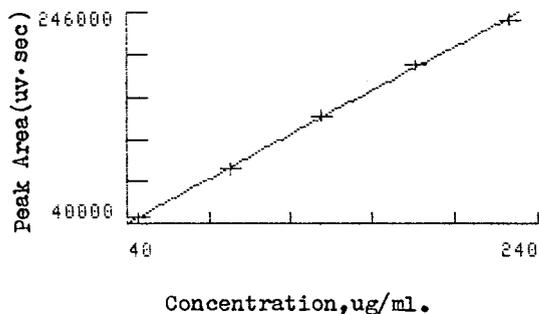
Fig. 3. Calibration graph for 4-nitrobenzoyl chloride. Column, Shim-Pack CLC-C<sub>3</sub> (150 × 4.6 mm I.D.); eluent, cyclohexane-THF (70/30, v/v); flow-rate, 1.0 ml/min; detection, UV at 300 nm.
