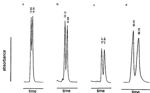
Fig. 4. Section of chromatograms of AQC-DL-alanine using the following chromatographic conditions: (a) 50% (v/v) methanol, 20°C, 0.5 ml/min; (b) 20% (v/v) methanol, 20°C, 0.7 ml/min; (c) 10% (v/v) methanol, 20°C, 0.8 ml/min; (d) 20% (v/v) methanol, 10°C, 0.5 ml/min.
