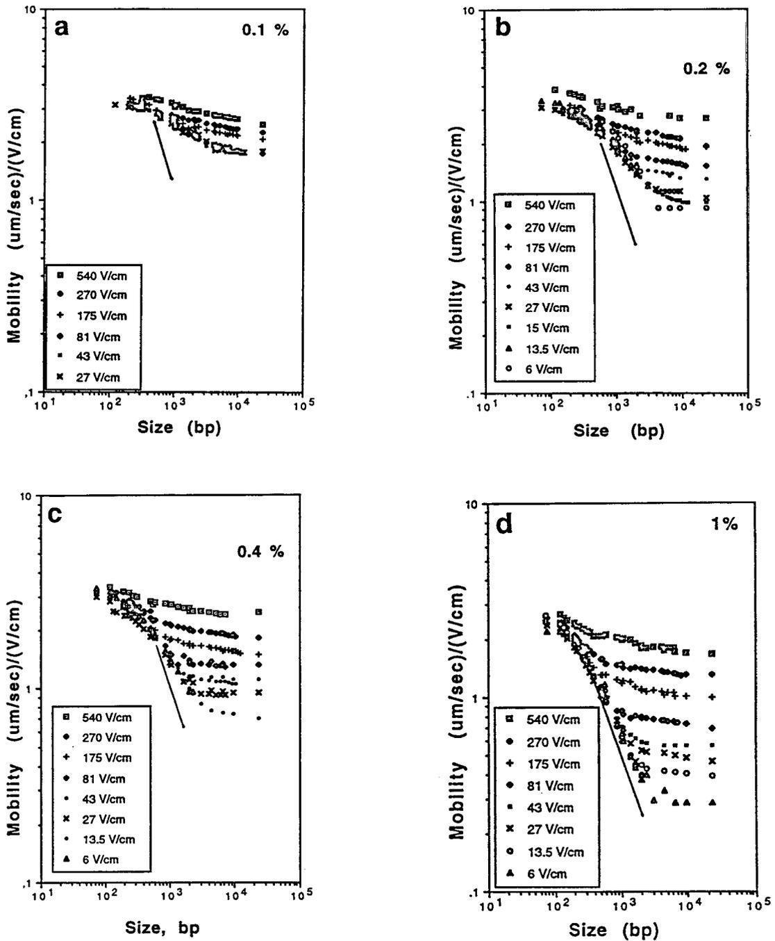
Fig. 4. Dependence of the electrophoretic mobility of linear double-stranded DNA fragments on the molecular mass in (a) 0.1, (b) 0.2, (c) 0.4 and (d) 1% HPC solutions at different electric field strengths in  $1 \times \text{TBE}$  containing  $10 \mu\text{M}$  ethidium bromide at  $25^\circ\text{C}$ . The lines have a slope of  $-1$ .
