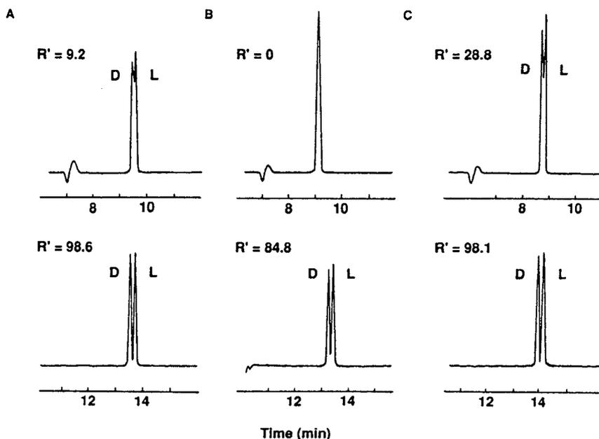
Fig. 1. Chiral separations of (A) dansyl-D,L- $\alpha$ -amino-*n*-butyrac acid, (B) dansyl-D,L-phenylalanine and (C) dansyl-D,L-serine with 10 mM  $\beta$ -CD before (upper traces) and after (lower traces) the addition of 7 M urea.
