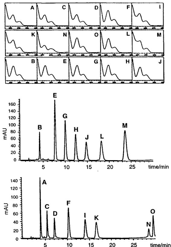
Fig. 2. Gradient HPLC–UV trace for sesquiterpene aryl esters A–O. For conditions, see Experimental. UV traces were recorded at 254 nm with UV spectra recorded from 170 to 400 nm. For peak identities, see Fig. 1.
