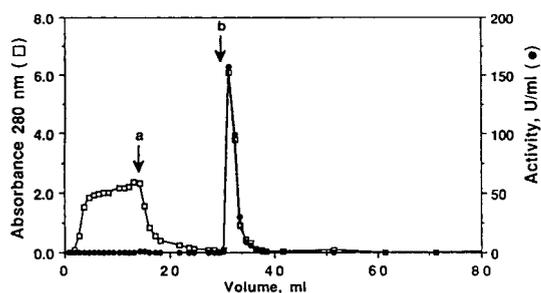
Fig. 5. LDH purification profile on Red Sepharose. Experimental conditions:  $1.2 \times 1.0$  cm I.D.; flow-rate 0.5 ml/min. The crude extract was applied to a column until breakthrough. The arrows indicate: a = washing after breakthrough with 20 mM Tris·HCl, pH 7.3; b = elution with 1% PEI-700 in 20 mM Tris·HCl, pH 7.3. The column was regenerated with 1% polyacrylate in 0.1 M glycine buffer pH 12 containing 1 M NaCl and reequilibrated with 20 mM Tris·HCl buffer pH 7.3.
