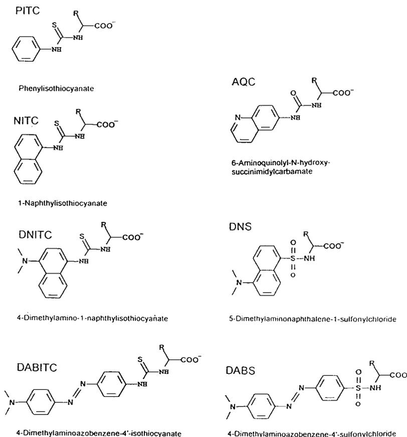
Fig. 1. Chemical structures of the amino acid derivatives investigated, R = amino acid side chain. Abbreviations refer to the reagents employed.
