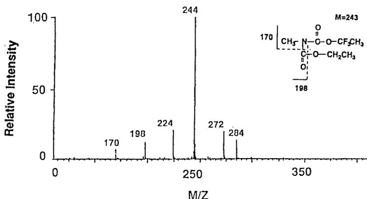
Fig. 3. Positive CI spectrum of derivatized sarcosine using methane as reagent gas. The  $m/z$  224, 244, 272, and 284 are  $[M - F]^+$ ,  $[M + H]^+$ ,  $[M + C_2H_5]^+$ , and  $[M + C_3H_5]^+$  peaks, respectively.
