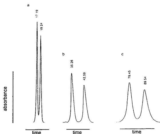
Fig. 2. Section of chromatograms of PITC-derivatized amino acids (a) DL-alanine, (b) DL-tryptophane, (c) DL-glutamic acid. Retention times in minutes. Flow-rate: 0.5 ml/min; eluent composition, aqueous buffer [0.1 M NH<sub>4</sub>Ac pH 6.5–MeOH (60:40, v/v)]. Other chromatographic conditions as specified in Experimental.
