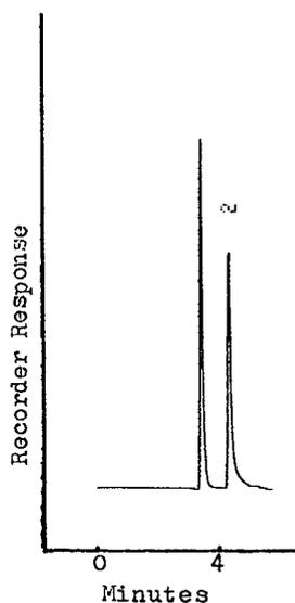
Fig. 2. Chromatogram of a mixture containing (1) 4-nitrobenzoyl chloride and (2) 4-nitrobenzoic acid. Column, Shim-Pack CLC-C<sub>3</sub> (150 × 4.6 mm I.D.); eluent, cyclohexane-THF (70/30, v/v); flow-rate, 1.0 ml/min; injection volume, 5 μl; detection, UV at 300 nm.
