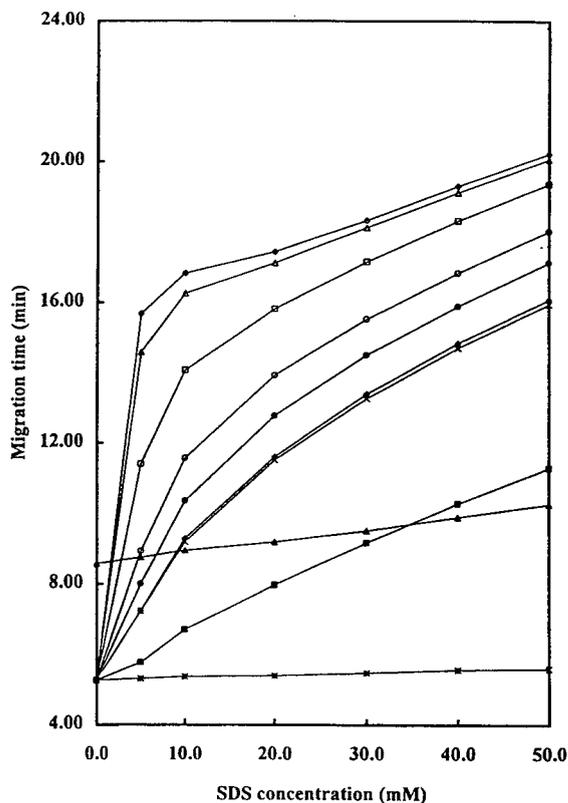
Fig. 3. Effect of SDS concentration on migration time. Electrophoretic medium: 0–50 mM SDS–15 mM  $\text{Na}_2\text{B}_4\text{O}_7$ –15 mM  $\text{NaH}_2\text{PO}_4$ . Capillary: 67.5 cm (59.5 cm to detector)  $\times$  50  $\mu\text{m}$  I.D. Applied voltage: 20 kV. Cartridge temperature: 30°C. Detection: UV at 200 nm. \* = EOF;  $\square$  = 1;  $\triangle$  = 2;  $\diamond$  = 3;  $\times$  = 4;  $\circ$  = 5;  $\circ$  = 6;  $\square$  = 7;  $\triangle$  = 8;  $\diamond$  = 9.
