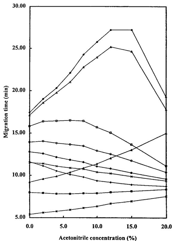
Fig. 4. Effect of  $\text{CH}_3\text{CN}$  concentration on migration time. Electrophoretic medium: mixture of 0–20%  $\text{CH}_3\text{CN}$  with a buffer of 20 mM SDS–15 mM  $\text{Na}_2\text{B}_4\text{O}_7$ –15 mM  $\text{NaH}_2\text{PO}_4$ . Other conditions and symbols as in Fig. 3.
