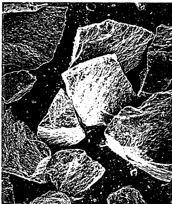
Fig. 1. Scanning electron micrograph of 50% graphite PFC particles. The individual particles are irregular in shape and exhibit characteristic dimensions in the range 74–149 μm.
