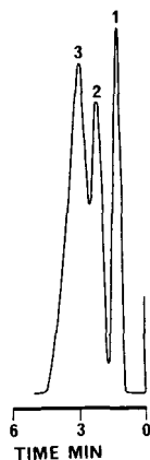
Fig. 1. Chromatogram of chlorpropamide (1), tolbutamide (2) and 1-isopentyl-3-( p -tolylsulphonyl)urea (3). Solvent system, acetonitrile—water (28:72, v/v).
