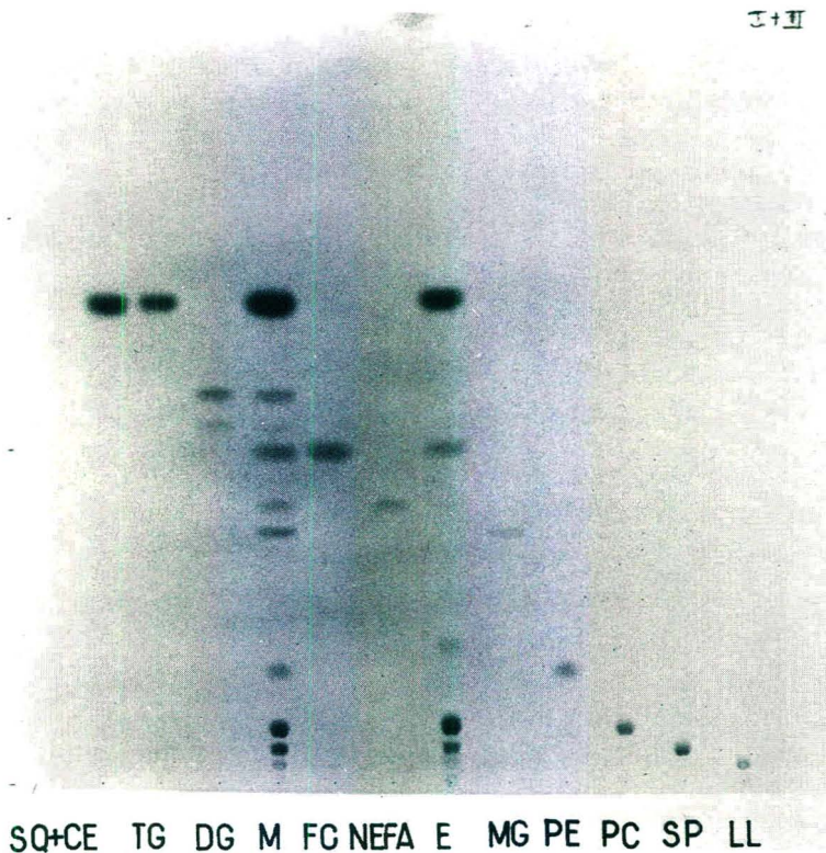
Fig. 1. Thin-layer chromatogram of lipids developed in solvent systems I + II. SQ = Squalene; CE = cholesterol ester; TG = triglycerides; DG = diglycerides (diglyceride 1,3 = 1,3DG and diglyceride 1,2 = 1,2DG); M = reference mixture of the twelve standard lipids; FC = free cholesterol; NEFA = non-esterified fatty acid; E = human serum lipid extract; MG = monoglyceride; PE = phosphatidyl ethanolamine; PC = phosphatidyl choline; SP = sphingomyelin; LL = lysolecithin.
