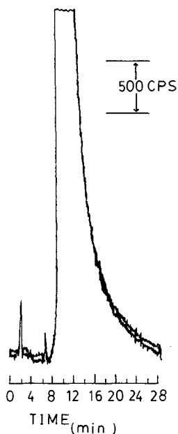
Fig. 3. Chromatogram of ^{99}\text{Mo}/^{99m}\text{Tc} generator eluent ( \approx 60 mCi/ml) with gamma-detection. Conditions: eluent 0.1 M acetate, pH 4.5; flow-rate 1.5 ml/min; temperature ambient.
