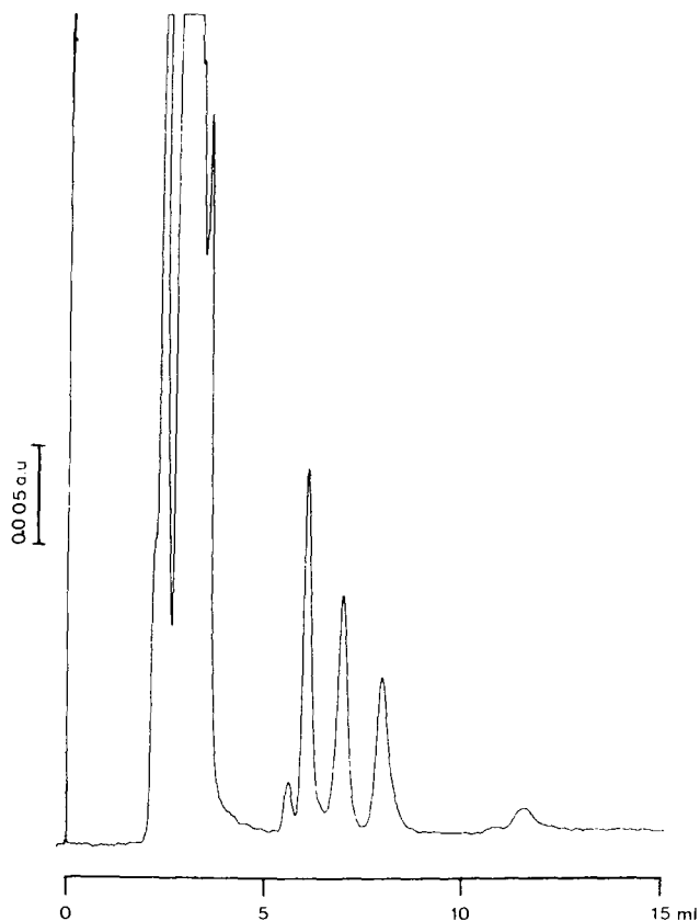
Fig. 9. LC trace of a concentrated diethyl ether extract from the patient of Fig. 8. Sample volume and other details as in Fig. 8. The trace shows chlorpromazine (8 ml), 7-hydroxy-chlorpromazine (7 ml), demonomethylchlorpromazine (6 ml) and chlorpromazine N-oxide (5.5 ml). The chlorpromazine concentration was 58.3 ng/ml. The metabolites are shown for identification only.
