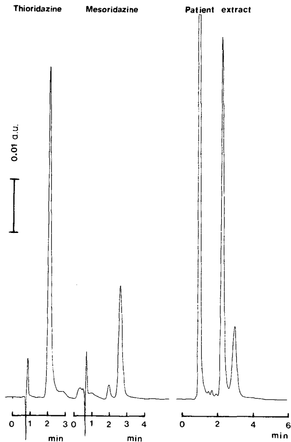
Fig. 10. LC trace of an investigation of a patient receiving thioridazine. The trace shows the drug and its metabolite as standards and in a hexane extract from plasma. The patient was receiving 200 mg thioridazine daily and the sample was collected 20 h post dosage. Detection by UV (254 nm); y axis in absorbance units. The thioridazine concentration was 26.1 ng/ml.
