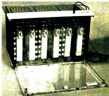
tions. Designed to meet the requirements of Anderson and Anderson ISO-DALT applications, the standard cell comes with enough spacers, plates, and accessories to run up to 12 two-dimensional slab gels. Three upper buffer chambers, which fit into a single large lower chamber, are used both to cast the gels and to support them during the electrophoresis. The large volume of the lower buffer is adequate for cooling two-dimensional SDS gels, so that no heat exchangers are needed.
