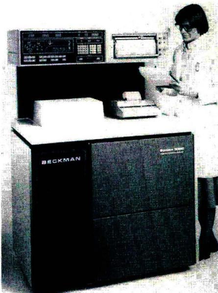
The System 6300 can quantitate samples of 20  $\mu$ l or less, containing 50 pmol or less of each component. The instrument can detect components in concentrations as low as 10 pmol. A touch-control panel provides micro-processor control at the operator's fingertips. Automatic program linking eliminates manual adjustments of preparation of the instrument prior to operation or between analytical programs. Four different programs can be stored in the instrument's memory.
