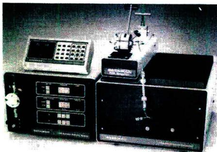
tem can be expanded and updated. The Spherogel columns provide rapid elution; they separate globular proteins with molecular weights ranging from 2000 to 1,000,000. Recommended accessories include a Kipp BD-40 recorder, a zinc lamp, a 214 nm filter, a pre-column and a table top centrifuge.
