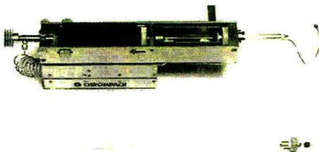
this tube are desorbed thermally in an oven. The second part is the cold trap, consisting of a piece of fused silica that can be cooled. In this part of the injector the components, thermally desorbed from the first part, condense in a very small volume. The cold trap is heated instantly and the components are injected as a very small band on the following fused-silica capillary column of the GC system. The injector can be used with most gas chromatographs currently available.
