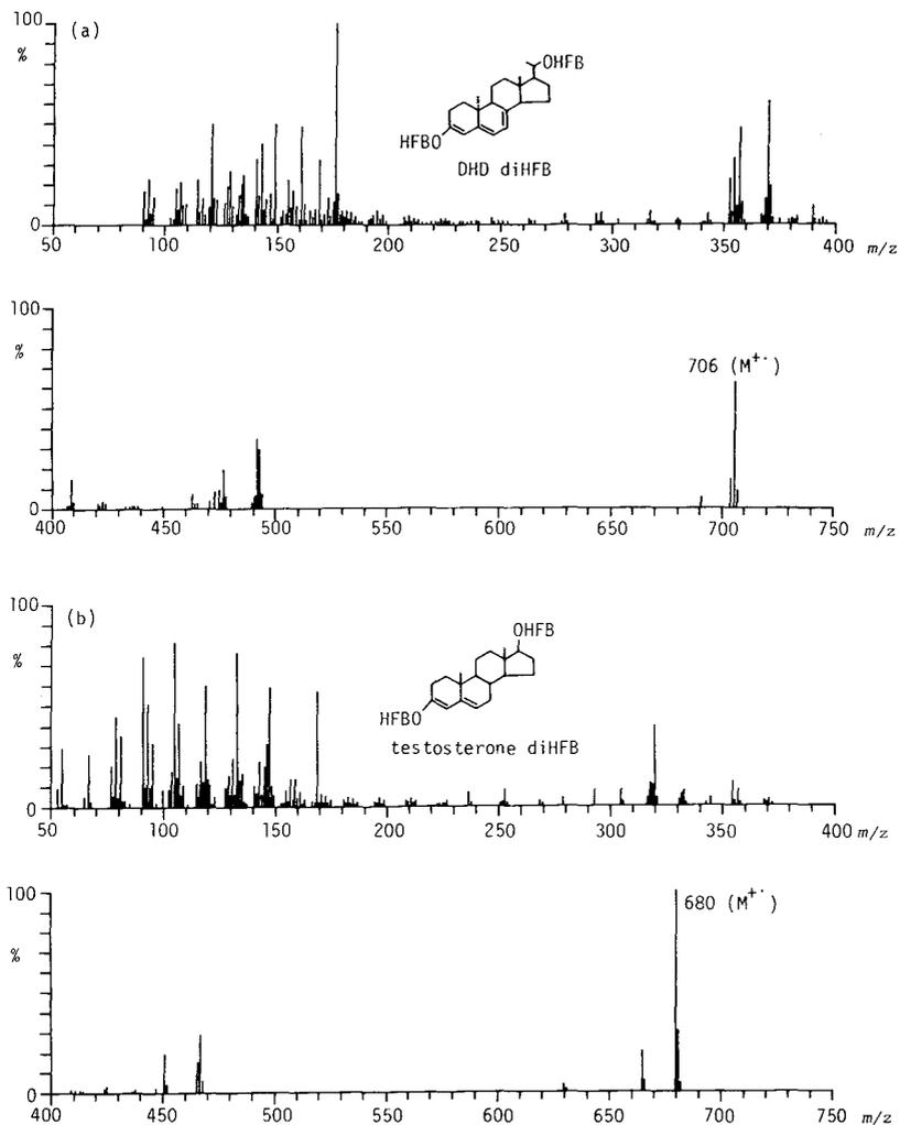
Fig. 2. Mass spectra of (a) DHD diHFBB and (b) testosterone diHFBB.
