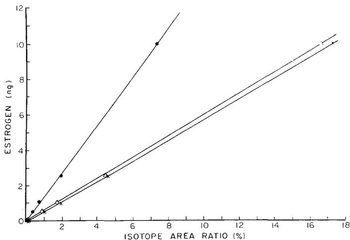
Fig. 4. Standard curves of estrogens: ( $\Delta$ — $\Delta$ ) estrone; ( $\times$ — $\times$ ) estradiol; ( $\bullet$ — $\bullet$ ) estriol. Isotope area ratio (%) was obtained by dividing the peak area of unlabelled estrogen by that of labelled estrogen.
