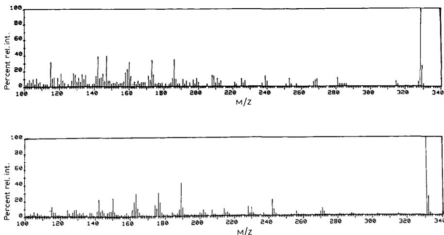
Fig. 2. Electron-impact (70 eV) mass spectra of estradiol methyl ether acetate (top), and 3-O-C<sup>2</sup>H<sub>3</sub>-estradiol acetate (bottom).
