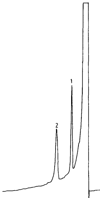
Fig. 1. Typical chromatogram obtained for the assay of urinary creatinine. Peaks: 1 = L-hydroxyproline standard (110 nmol); 2 = creatinine (38 nmol).
