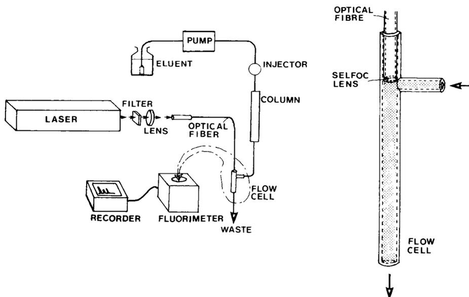
Fig. 1. Schematic diagram of the experimental system for HPLC with laser fluorimetric detection. The argon laser beam transmits along an optical fibre which is axially introduced into a flow cell system to excite the fluorophores of a flowing sample in a capillary cell, without irradiating the cell walls and/or the liquid surface.
