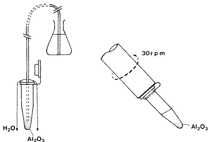
Fig. 2. Schematic diagram of the CA pre-treatment method. Right: to mix the alumina with Tris-HCl buffer or OPA solution, the Eppendorf tube attached on the rotary rod was rotated at a constant rate (30 rpm). Left: to wash the alumina with water, the water, which was continuously flowing through the PTFE tube, was circulated in the Eppendorf tube. The water, but not the alumina, overflowed from the tube and fresh water was applied constantly to the tube from the water reservoir.
