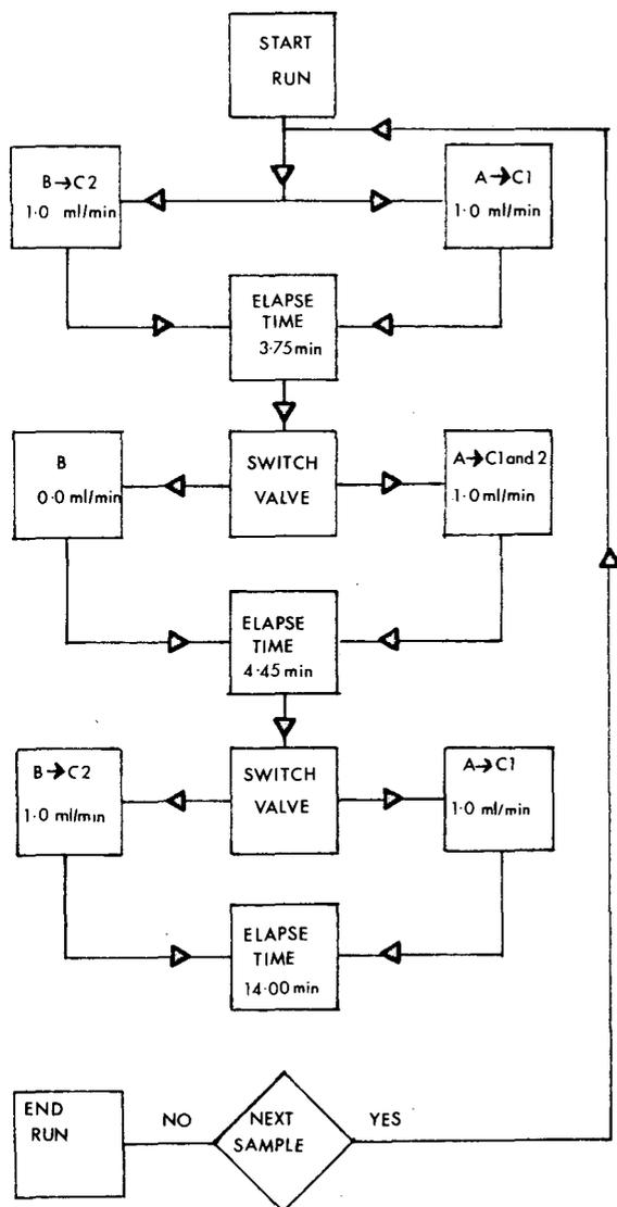
Fig. 4. Summary of the switching events for the analysis of TCAR in plasma. A, B, C1 and C2 refer to pumps A and B, column 1 (Hypersil) and column 2 (ODS Hypersil or  $\mu\text{Bondapak C}_{18}$ ), respectively. The arrows ( $\rightarrow$ ) within the boxes indicate the flow from the respective pumps through the columns. The elapse times are from the point of injection. See Fig. 3 for further details.
