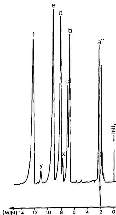
Fig. 5. Chromatogram of a plasma extract from a patient receiving a 600-mg oral dose of bamifylline (Trentadil) for three months and spiked with 1.25 \mu\text{g/ml} of fenetylline (internal standard). Chromatographic conditions are described in Table I [3]. a'' = caffeine, b = AC 85, c = AC 155, d = bamifylline, e = AC 119, f = fenetylline, x and y = unknown peaks (minor metabolites?).
