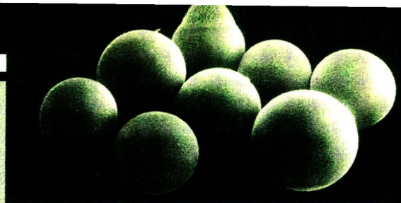
SEM photomicrograph of VYDAC HS silica.
