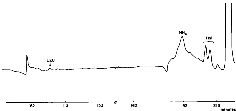
Fig. 4. Amino acid analyzer chromatogram of the same fraction as in Fig. 3 after it had been subjected to acid hydrolysis in 2 M hydrochloric acid for 4 h at 109°C and brought to pH 3 with 4 M lithium hydroxide. Curve represents the sum of the absorptions at 440 and 570 nm. Only sections of interest of the chromatogram are shown. Abscissa: retention times in min; ordinate: absolute units proportional to optical density. Size of sample: 200 \mu l; recorder set at highest sensitivity.
