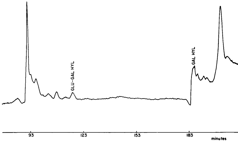
Fig. 5. Amino acid analyzer chromatogram of the same sample as in Fig. 3 but done under the final parameters chosen for this method. Only the section of interest of the chromatogram is shown. Curve represents the sum of the absorptions at 440 and 570 nm. Abscissa: retention times in min; ordinate: absolute units proportional to optical density; size of sample: 625 \mu\text{l} ; recorder set at highest sensitivity (0.1 absorption).
