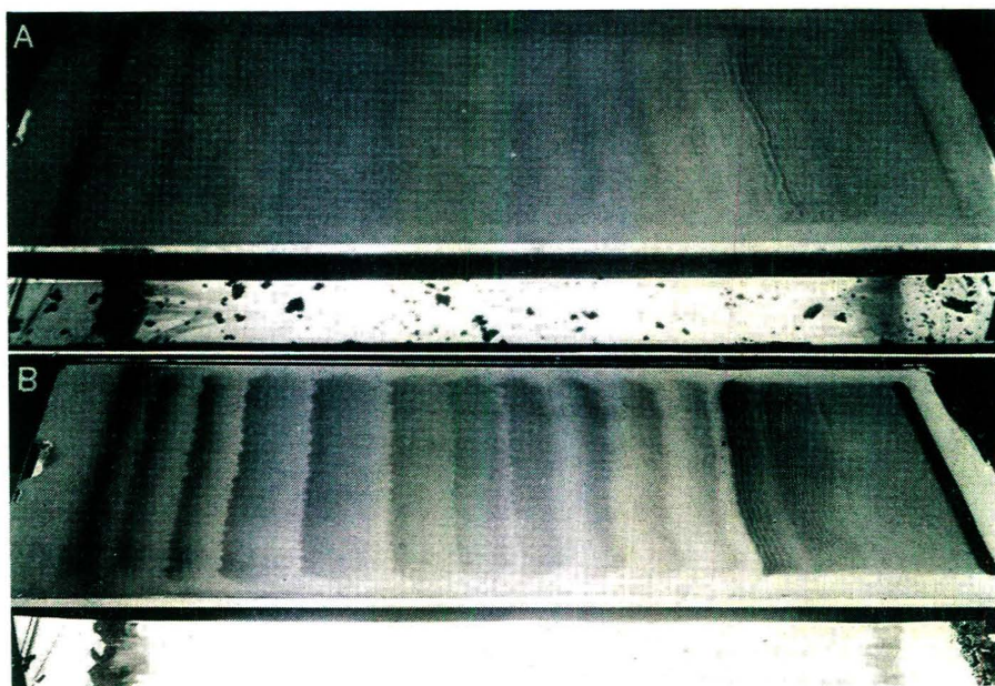
Fig. 1. (A). Developed thin-layer chromatogram exposed to iodine vapors. A 6 mg sample of malto-oligosaccharides was separated as described for the large plates in Table II. (B). The plate pictured in (A) after spraying with 20 ml of detection reagent (18 ml of 95% ethanol, 1.0 ml concentrated H_2SO_4 and 1.0 ml of anisaldehyde) and heating at 100° for 25 min 4 .
