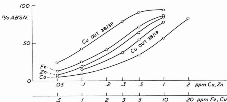
FIG. 3. Curves percent absorption vs. log concentration for Cu, DU<sup>®</sup>-2, and turbulent flow burner (3 Burners/3 Passes); Cu, DU<sup>®</sup>-2, and turbulent flow burner (3 Burners/1 Pass); Zn, Fe, Ca, same conditions as shown in Fig. 2.
