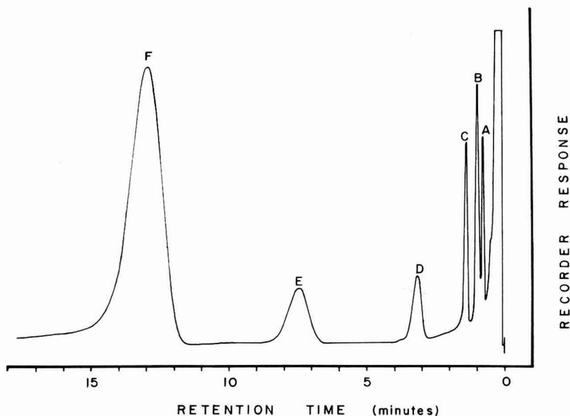
FIG. 1. Separation of alkaloids. A, Caffeine, 50 ng; B, cocaine, 50 ng; C, atropine, 50 ng; D, codeine, 0.1  $\gamma$ ; E, heroin, 1  $\gamma$ ; F, morphine, 5  $\gamma$ . Conditions: 3-foot glass column (1/8 inch o.d.) packed with Hi-Eff-8B 1% on 100/120 mesh silanized Gas Chrom P. Oven temperature 220°C; injector 275°C. Flow rate of carrier gas (nitrogen) 60 ml/minute. Input impedance 10<sup>9</sup> ohms; output sensitivity 1  $\times$ ; attenuation 4  $\times$ .
