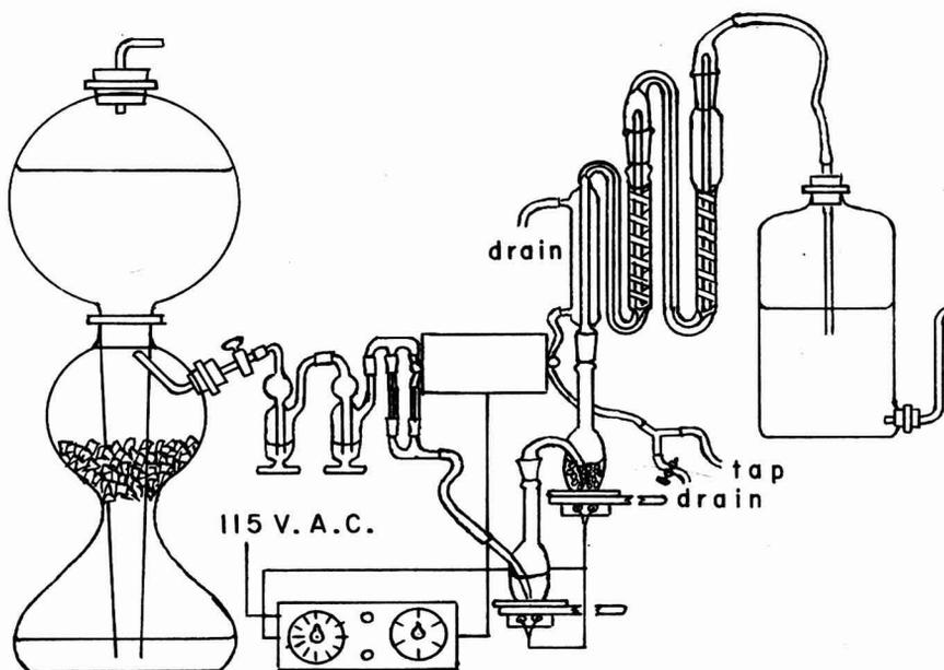
FIG. 1. Semiautomated alkoxy apparatus.
