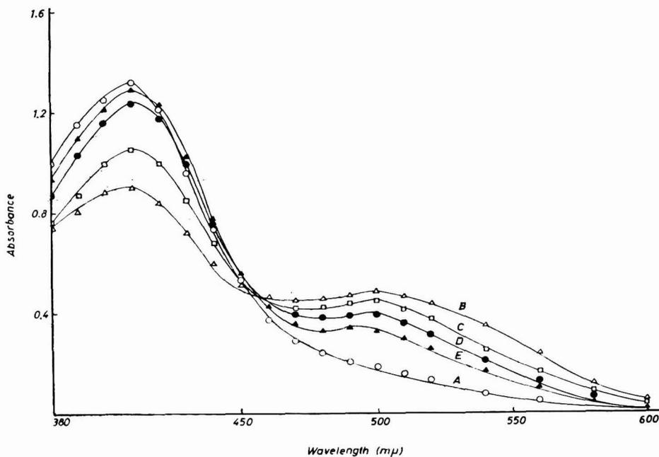
FIG. 3. Absorption spectra of tantalum-PAR chelate, pH 6.0. Curve A: Reagent  $c = 8.0 \times 10^{-5}M$ ; Curve B:  $c = 16.0 \times 10^{-5}M$ ,  $p = 0.5$ ; Curve C:  $c = 8.0 \times 10^{-5}M$ ,  $p = 1.0$ ; Curve D:  $c = 4.0 \times 10^{-5}M$ ,  $p = 2.0$ ; Curve E:  $c = 2.67 \times 10^{-5}M$ ,  $p = 3.0$  ( $p = c'/c$ ).
