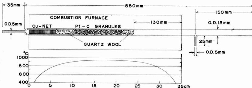
FIG. 3. Thermal decomposition tube.
