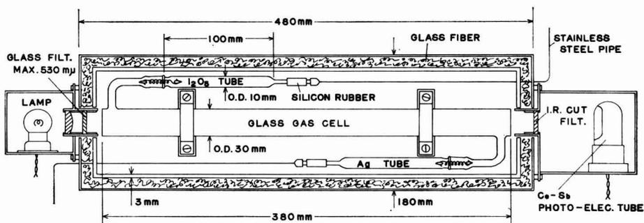
FIG. 4. Carbon monoxide measuring system.
