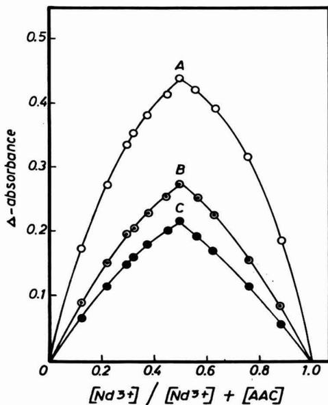
FIG. 3. Determination of the composition of neodymium-AAC chelate by the method of continuous variations using equimolecular solutions at pH 6.0 at 550 m $\mu$ . Concentrations in Curve A =  $4.0 \times 10^{-4}M$ ; Curve B =  $2.0 \times 10^{-4}M$ ; Curve C =  $1.33 \times 10^{-4}M$ .  $P = 1$ .
