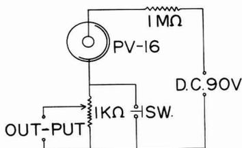
FIG. 5. Photoelectric circuit.
