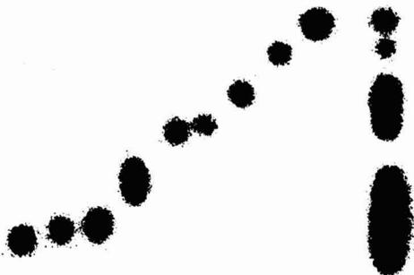
FIG. 2. Separation of a mixture of primary, secondary, and tertiary alcohol esters of pyruvic acid 2,6-dinitrophenylhydrazone into classes by TLC on magnesium oxide. Solvent, benzene:  $\text{CHCl}_3$  (3:1). Diagonally from top to bottom: tert  $\text{C}_8$ , tert  $\text{C}_4$ , tert  $\text{C}_5$ , sec  $\text{C}_{18}$ , sec  $\text{C}_4$ , sec  $\text{C}_3$ , pri  $\text{C}_{18}$ , pri  $\text{C}_2$ , pri  $\text{C}_1$ . Column on right represents a mixture of all of the compounds.
