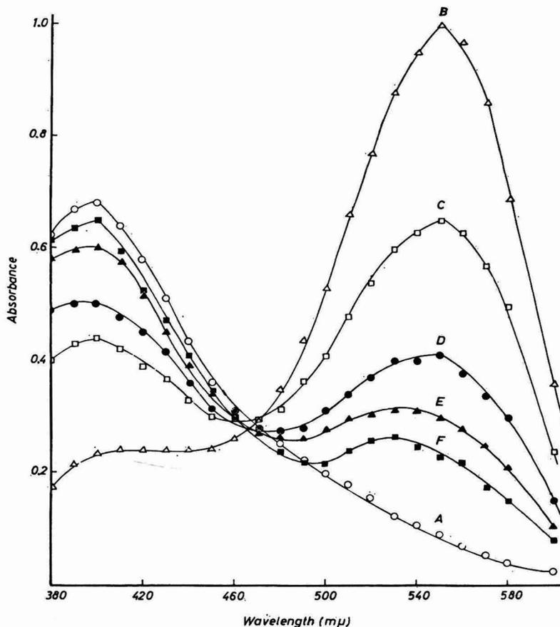
FIG. 1. Absorption spectra of vanadium-PAR chelate, pH 5.0. Curve A: Reagent,  $c = 4.0 \times 10^{-5}M$ ; Curve B:  $c = 8.0 \times 10^{-5}M$ ,  $p = 0.5$ ; Curve C:  $c = 4.0 \times 10^{-5}M$ ,  $p = 1.0$ ; Curve D:  $c = 2.0 \times 10^{-5}M$ ,  $p = 2.0$ ; Curve E:  $c = 1.33 \times 10^{-5}M$ ,  $p = 3.0$ ; Curve F:  $c = 1.0 \times 10^{-5}M$ , ( $c = \text{conc. of metal ion and } c' = \text{conc. of reagent, } p = c'/c$ ).
