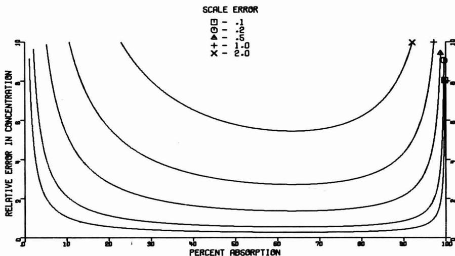
FIG. 1. Relative error in concentration as a function of percent absorption at different values of scale error. This figure is a direct reproduction of the automatic plotting obtained from computer data.
