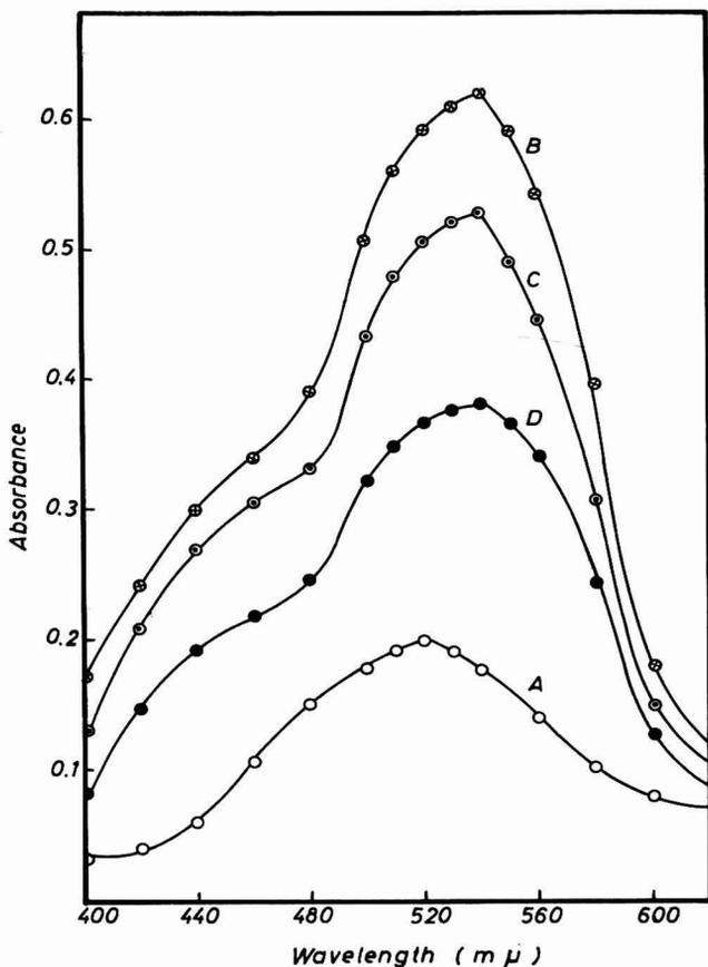
FIG. 1. Absorption spectra of neodymium-AAC chelate. Curve A, AAC =  $1.6 \times 10^{-4}M$ . Curve B, AAC =  $1.6 \times 10^{-4}M$ ;  $NdCl_3 = 3.2 \times 10^{-4}M$ . Curve C, AAC =  $1.6 \times 10^{-4}M$ ;  $NdCl_3 = 1.6 \times 10^{-4}M$ . Curve D, AAC =  $1.6 \times 10^{-4}M$ ;  $NdCl_3 = 8.0 \times 10^{-5}M$ .
