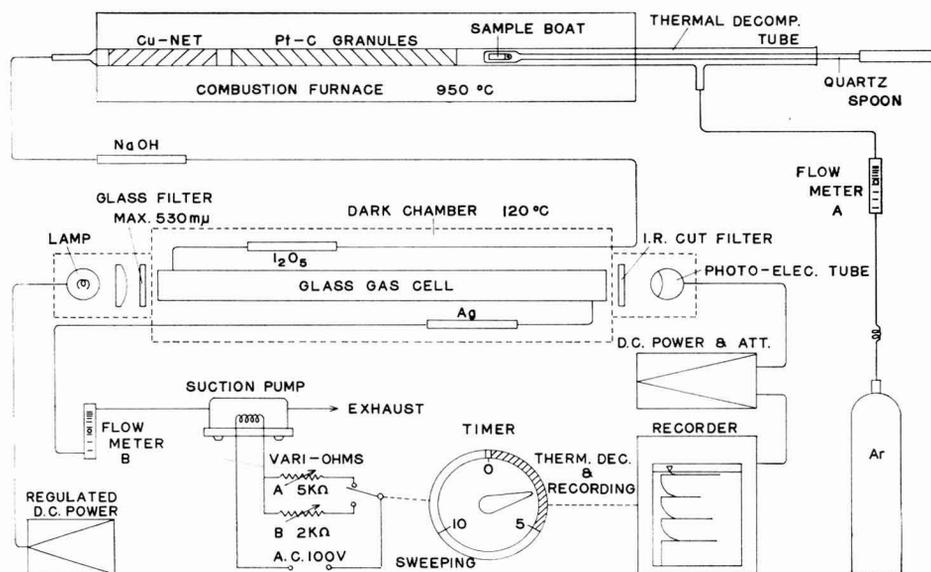
FIG. 1. Schematic diagram of oxygen analyzer.
