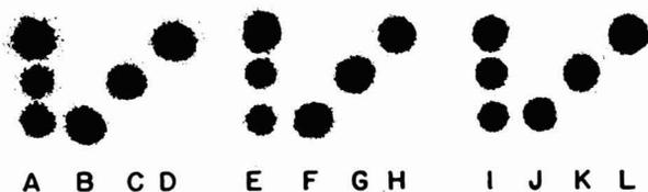
FIG. 3. Separation of isomeric alcohol esters of pyruvic acid 2,6-dinitrophenylhydrazone on aluminum oxide G. Solvent, methyl cyclohexane:diethylamine (65:35). (A) Top to bottom: tert  $C_6$ , sec  $C_6$ , pri  $C_6$ ; (B) pri  $C_6$ ; (C) sec  $C_6$ ; (D) tert  $C_6$ ; (E) Top to bottom: tert  $C_7$ , sec  $C_7$ , pri  $C_7$ ; (F) pri  $C_7$ ; (G) sec  $C_7$ ; (H) tert  $C_7$ ; (I) Top to bottom: tert  $C_8$ , sec  $C_8$ , pri  $C_8$ ; (J) pri  $C_8$ ; (K) sec  $C_8$ ; (L) tert  $C_8$ .
