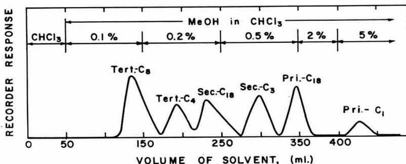
FIG. 1. Separation of a mixture of primary (pri), secondary (sec), and tertiary (tert) alcohol esters of pyruvic acid 2,6-dinitrophenylhydrazone into classes by column chromatography on magnesium oxide.
