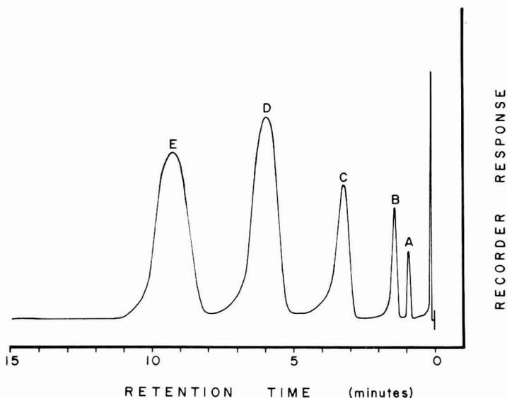
FIG. 1. Separation of pesticides. A, Aldrin, 1 ng; B, Lindane, 0.2 ng; C, Dieldrin, 5 ng; D, Morocide, 20 ng; E, *p-p'*-DDT 25 ng. Conditions: 3-foot glass column ( $\frac{3}{8}$  inch o.d.) packed with Hi-Eff-8B 1% on 100/120 mesh silanized Gas Chrom P. Oven temperature 190°C; injector 275°C. Detector: Electron capture. Flow rate of carrier gas (nitrogen) 40 ml/minute. Input impedance  $10^7$  ohms; output sensitivity  $1 \times$ ; attenuation  $4 \times$ .
