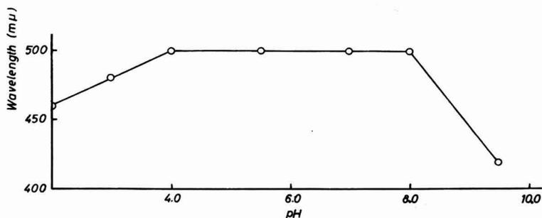
FIG. 6. Variation of  $\lambda_{\max}$  with pH of tantalum-PAR system. Conc. of tantalum = PAR =  $8.0 \times 10^{-5}M$ .
