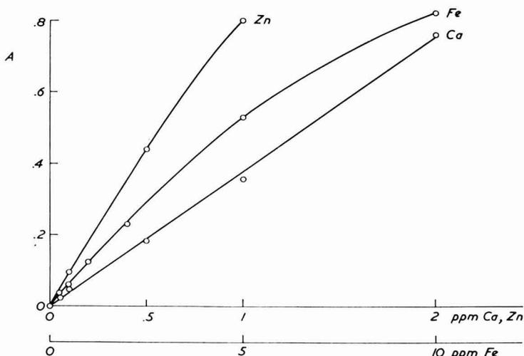
FIG. 2. Working curves, absorbance vs. concentration for Zn, DU<sup>®</sup>-2, and turbulent flow burner (3 Burners/3 Passes); Fe, DU<sup>®</sup>-2, and turbulent flow burner (3 Burners/3 Passes); Ca, DB<sup>®</sup> and laminar flow burner (1 Pass).
