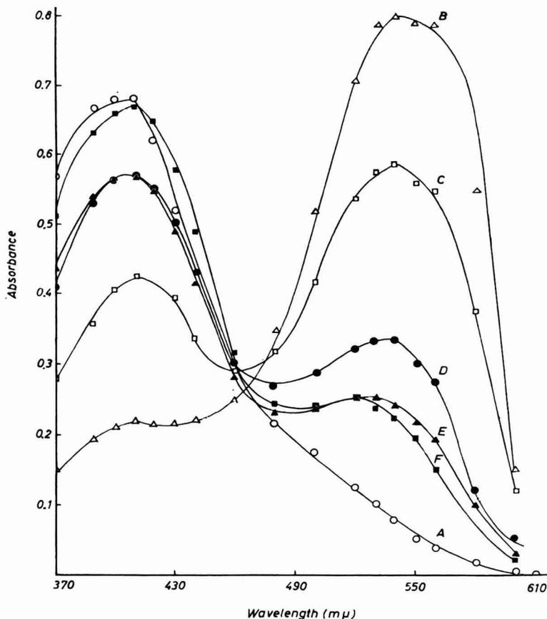
FIG. 2. Absorption spectra of niobium-PAR chelate, pH 6.0. Curve A: Reagent,  $c = 4.0 \times 10^{-5}M$ ; Curve B:  $c = 8.0 \times 10^{-5}M$ ,  $p = 0.5$ ; Curve C:  $c = 4.0 \times 10^{-5}M$ ,  $p = 1.0$ ; Curve D:  $c = 2.0 \times 10^{-5}M$ ,  $p = 2.0$ ; Curve E:  $c = 1.33 \times 10^{-5}M$ ,  $p = 3.0$ ; Curve F:  $c = 1.0 \times 10^{-5}M$ ; ( $p = c'/c$ ).
