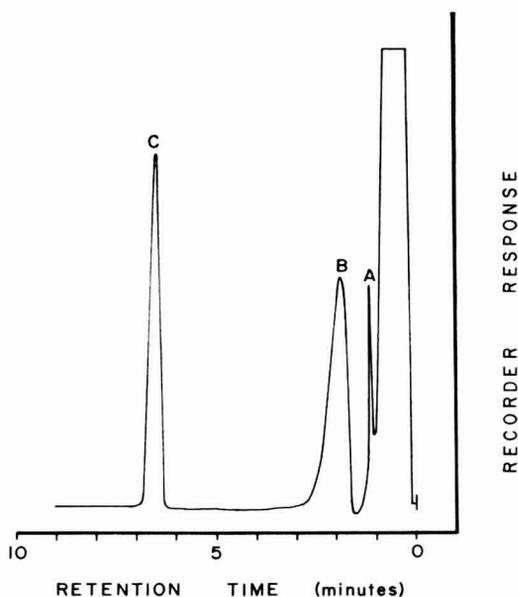
Fig. 3. Separation of tranquilizers. A, Meprobamate, 0.1  $\gamma$ ; B, reserpine, 5  $\gamma$ ; C, librium, 2  $\gamma$ . Conditions: 3-foot glass column ( $\frac{1}{8}$  inch o.d.) packed with Hi-Eff-8B 1% on 100/120 mesh silanized Gas Chrom P. Oven temperature 250°C; injector 275°C. Flow rate of carrier gas (nitrogen) 14.6 ml/minute. Input impedance 10<sup>9</sup> ohms; output sensitivity 1  $\times$ ; attenuation 4  $\times$ .
