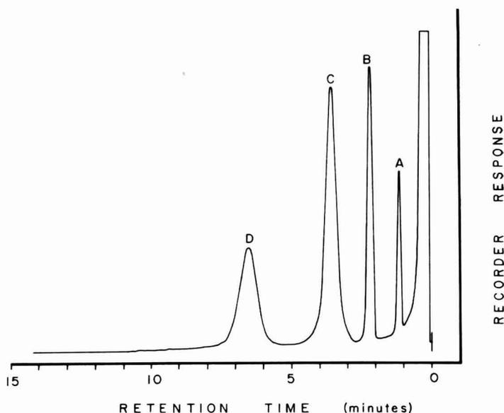
FIG. 2. Separation of alkaloids. A, Codeine, 0.1  $\gamma$ ; B, heroin, 1  $\gamma$ ; C, morphine, 2  $\gamma$ ; D, quinine, 2  $\gamma$ . Conditions: Same as in Fig. 1, except oven temperature 250°C. Flow rate of carrier gas (nitrogen) 54.4 ml/minute.
