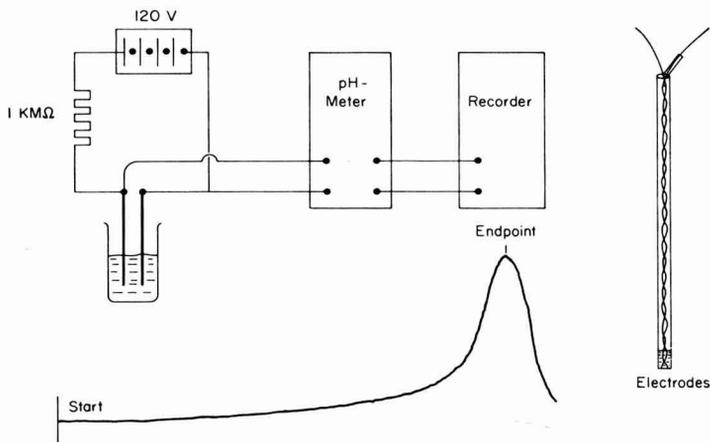
FIG. 2. Layout of titration setup, electrodes and titration curve. Even sharper end points were recently obtained with a 40-V battery instead of that with 120-V tension.
