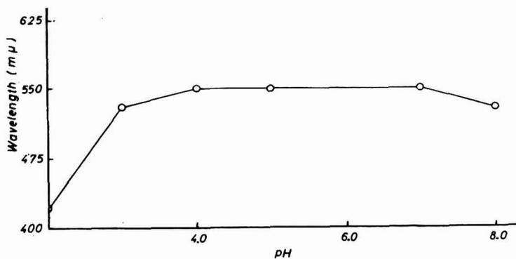
FIG. 4. Variation of  $\lambda_{\max}$  with pH of vanadium-PAR system. Conc. of vanadium = PAR =  $4.0 \times 10^{-5}M$ .
