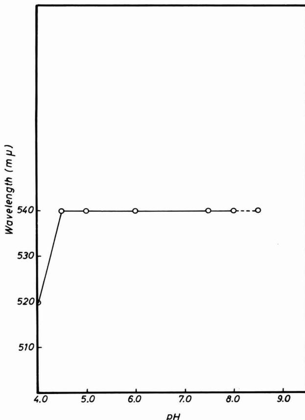
FIG. 2. Variation of  $\lambda_{\max}$  of neodimium-AAC chelate with pH. Final concentration of AAC =  $8.0 \times 10^{-5}M$ . Final concentration of  $NdCl_3$  =  $8.0 \times 10^{-5}M$ .
