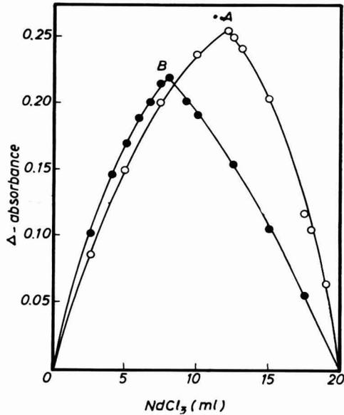
FIG. 7. Evaluation of stability constants by the method of continuous variations using nonequimolecular solutions at pH 6.0 at 550  $m\mu$ . Curve A AAC =  $4.0 \times 10^{-4}M$ ;  $NdCl_3 = 2.0 \times 10^{-4}M$ . Curve B AAC =  $2.0 \times 10^{-4}M$ ;  $NdCl_3 = 4.0 \times 10^{-4}M$ .
