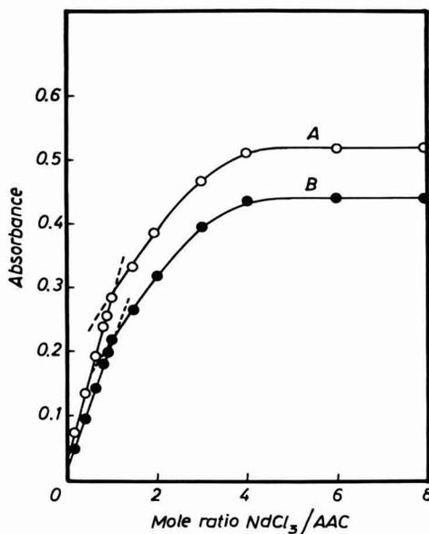
FIG. 4. Determination of the composition of neodymium-AAC chelate using mole ratio method at pH 6.0 at 550 m $\mu$ . Final concentration of AAC Curve A =  $1.0 \times 10^{-4}M$ . Curve B =  $8.0 \times 10^{-5}M$ .
