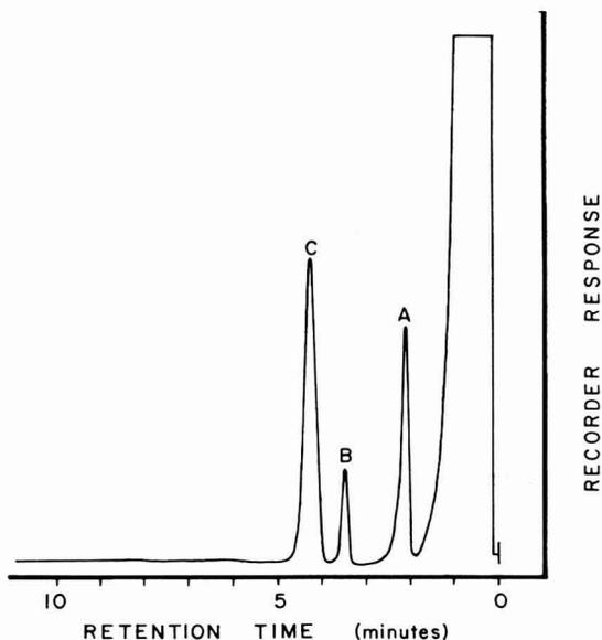
FIG. 2. Separation of tranquilizers. A, Triflupromazine, 2  $\gamma$ ; B, meprobamate, 0.1  $\gamma$ ; C, frenquel 1  $\gamma$ . Conditions: 3-foot glass column ( $\frac{1}{8}$  inch o.d.) packed with Hi-Eff-8B 1% on 100/120 mesh silanized Gas Chrom P. Oven temperature 220°C; injector 275°C. Flow rate of carrier gas (nitrogen) 15.8 ml/minute. Input impedance  $10^9$  ohms; output sensitivity 1  $\times$ ; attenuation 4  $\times$ .
