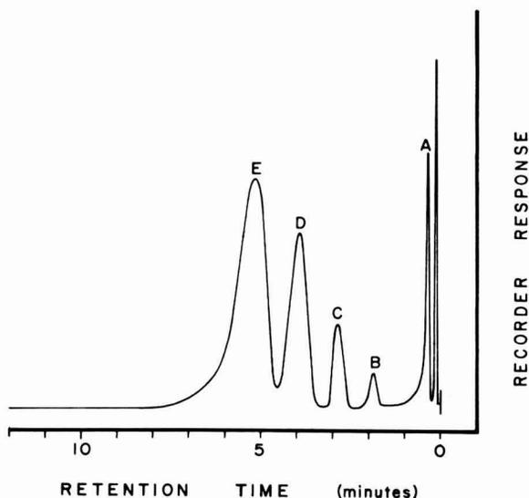
FIG. 2. Separation of pesticides. A, Trithion, 10 ng; B, Malathion, 10 ng; C, Parathion, 20 ng; D, Endrin, 10 ng; E, Ethion, 25 ng. Conditions: 3-foot glass column ( $\frac{1}{8}$  inch o.d.) packed with Hi-Eff-8B 1% on 100/120 mesh silanized Gas Chrom P. Oven temperature 190°C; injector 275°C. Detector: Electron capture. Flow rate of carrier gas (nitrogen) 40 ml/minute. Input impedance  $10^7$  ohms; output sensitivity  $1 \times$ ; attenuation  $4 \times$ .
