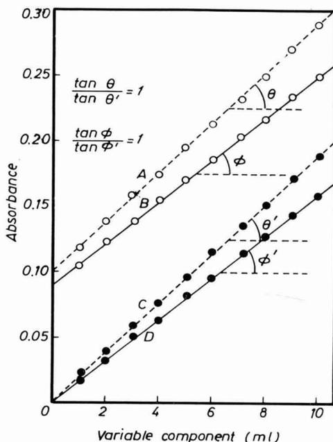
FIG. 5. Determination of the composition of AAC chelate of neodymium by the slope ratio method at pH 6.0. 10.0 ml ( $5.0 \times 10^{-4}M$ ) excess component + x ml ( $1.67 \times 10^{-4}M$ ) variable component + 5 ml ( $0.5M$ ) mannitol + (10 - x) ml  $H_2O$ . Curve AB = AAC in excess,  $NdCl_3$  varying. Curve CD =  $NdCl_3$  in excess, AAC varying. Broken lines = 550 m $\mu$ . Solid lines = 560 m $\mu$ .
