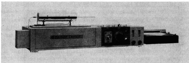
FIG. 2. Assembled oxygen analyzer.
