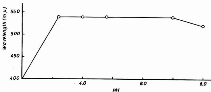
FIG. 5. Variation of  $\lambda_{\max}$  with pH. Niobium-PAR system. Conc. of niobium = PAR =  $4.0 \times 10^{-5}M$ .
