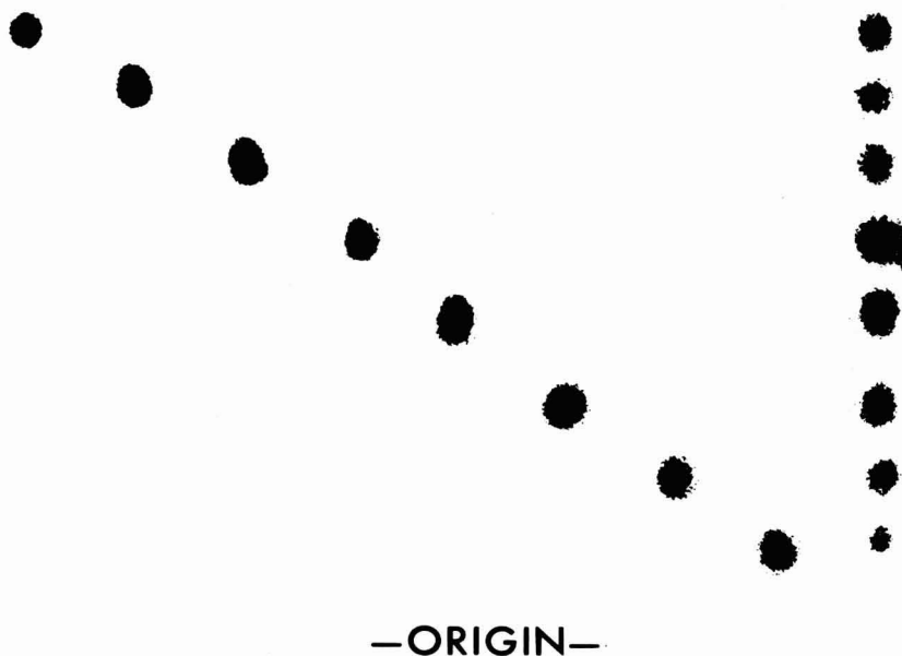
FIG. 5. Separation of primary amine 2,6-dinitrophenylhydrazones by reversed-phase partition chromatography. Support-Microcel T-38; stationary phase—mineral oil; mobile phase—acetonitrile: H_2O (3:1). Diagonally from top to bottom C_{11} through C_{18} primary amine derivatives. Column at right represents mixture of the 8 derivatives.
