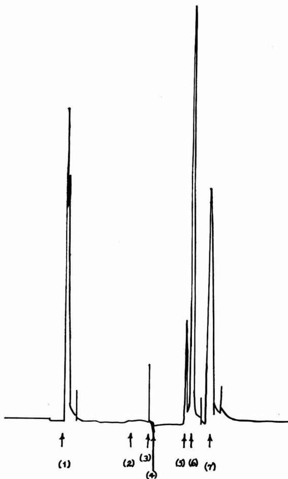
FIG. 1. Standard chromatogram. (1) Rod with sample and catalyst inserted into instrument cold zone; (2) purge peak; (3) oxidation combustion tube sealed off and sample inserted into hot oxidation combustion tube; (4) oxidation products injected into reduction combustion tube and then to GLC; (5) N_2 peak att. = 8; (6) CO_2 peak att. = 32; and (7) H_2O peak att. = 8.
