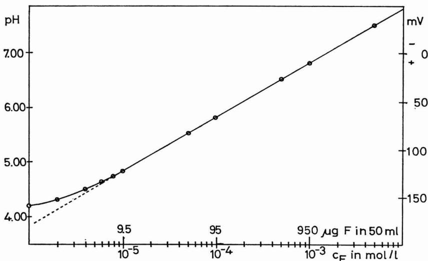
FIG. 1. Calibration curve for the electrode response in pH or mV mode of the instrument vs. fluoride ion concentration moles/liter or  $\mu\text{g}$  of F in 50 ml. Measurements were made in a TISAB background at  $24^\circ\text{C}$ , sample volume 50 ml.
