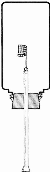
FIG. 1. Polypropylene oxygen combustion flask.
