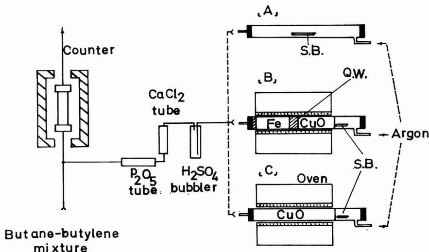
FIG. 1. Schematic representation of the apparatus used in the differential estimation of  $^3H$ ,  $^{14}C$ , and  $^{35}S$  in multilabeled organic samples: S.B. = sample boat; Q.W. = quartz wool.
