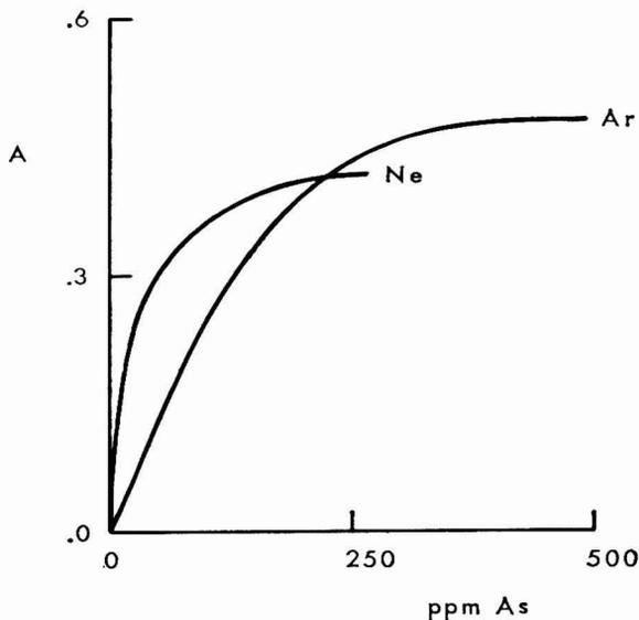
FIG. 2. Analytical calibration curves for arsenic (As 1937 Å) obtained with a Beckman Model 979 atomic absorption spectrophotometer and laminar flow burner (air-acetylene flame). With a neon filled lamp (Ne) better percentual sensitivity is obtained than with an argon filled lamp (Ar). However, loss of linearity is shown earlier in the case of the neon lamp because of the proximity of neon lines in that particular wavelength range.
