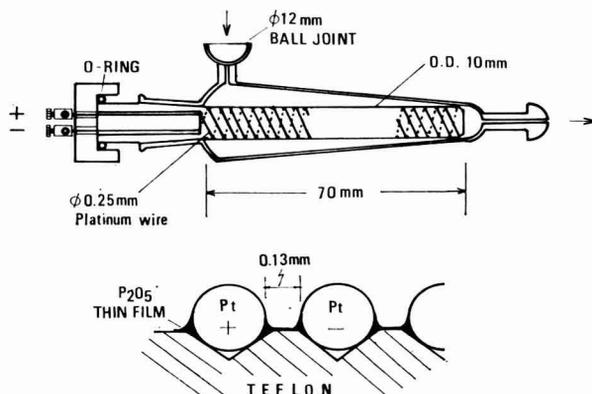
FIG. 2. Electrolytic cell and detail of electrode.
