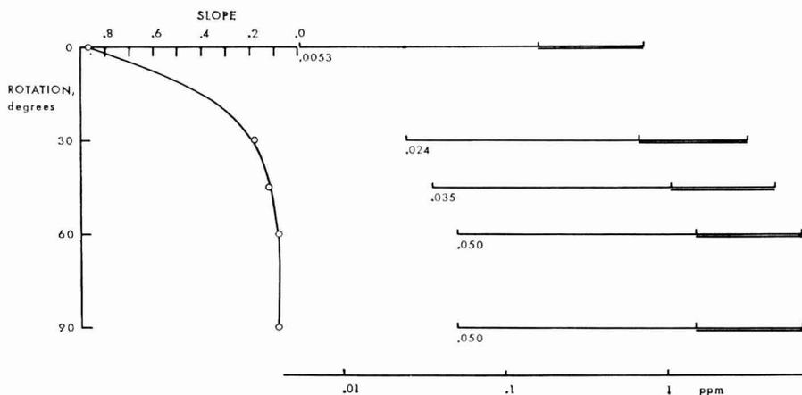
FIG. 3. Variation of dynamic concentration ranges as a function of the rotation angle of the laminar flow burner; data obtained for magnesium using a Beckman DU-2 Spectrophotometer with atomic-absorption accessory.
