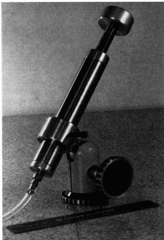
FIG. 1. The large capacity stainless steel syringe control: photograph of the unit mounted in an inclined position; schematic diagram showing (A) aluminum knob; (B) knob bonded to brass screw by epoxy cement; (C) \frac{1}{2} inch-13 N.C. threaded brass screw; (D) aluminum end-cap, \frac{1}{2} inch-13 N.C. inside, \frac{7}{8} inch-32 outside; (E) stainless steel tube polished inside, \frac{7}{8} inch i.d. \times 1.0 inch o.d.; (F) water reservoir above plunger; (G) tripod clamp support; (H) plunger fastened to brass screw by binding of threads; (I) baffle groove filled with grease; (J) Teflon plunger; (K) threads sealed with epoxy cement; (L) Luer-Lok connection (male), (M) aluminum end-cap, \frac{7}{8} inch-32 outside.
