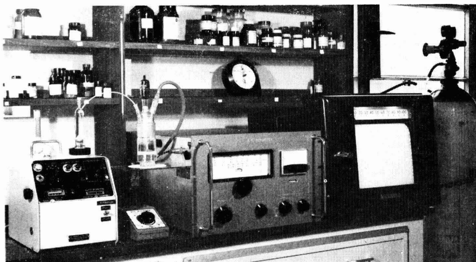
FIG. 2. View of the automatic titrimer (the rubber-tubing arrangement leads inert gas into the cell when required).
