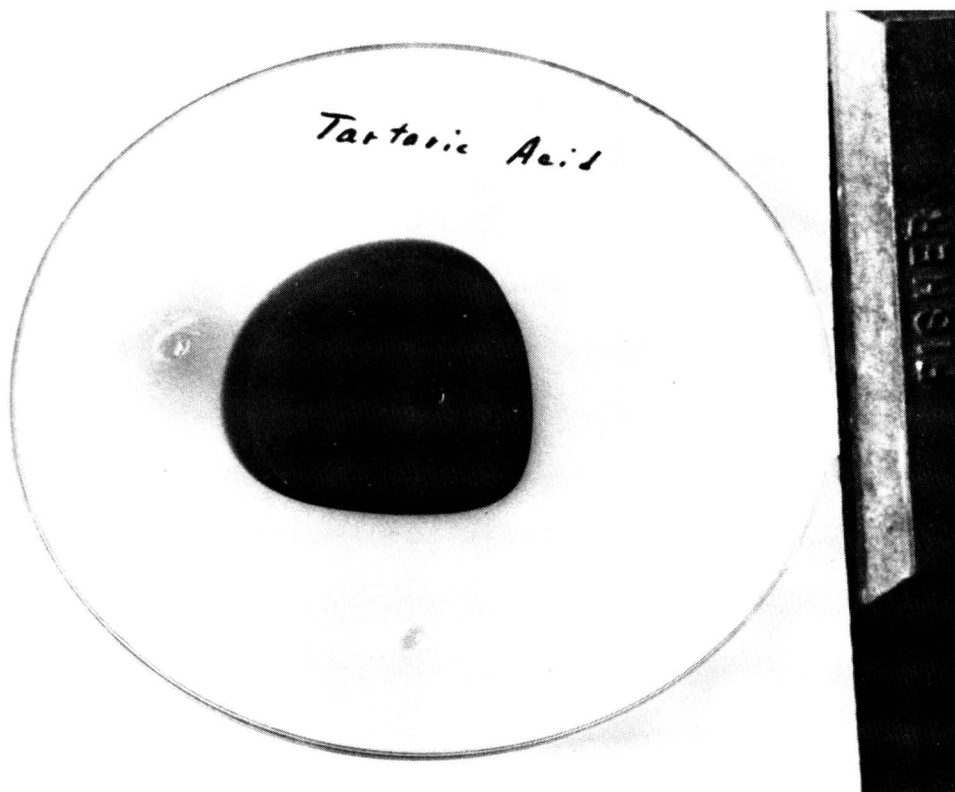
FIG. 3. Same as Plate II with tartaric acid instead of oxalic acid. There was some diffusion but no rings were formed with any of the ions.
