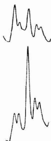
FIG. 2. Relative concentrations of peaks in the 50 min section of a gas chromatogram, before (upper chromatogram) and after subfractionation by silica gel in a 2 mm i.d. glass capillary.
