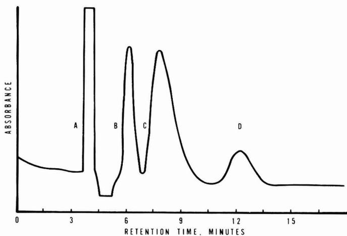
FIG. 3. HPLC chromatogram of pH 12 aqueous sample (Differential uv detector—254 nm). A. Sample matrix; B. triazole (1 mg/liter); C. excess DANH<sup>+</sup>; D. DANSe (3 mg/liter).
