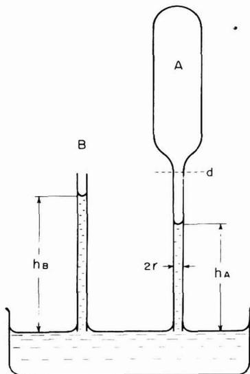
FIG. 2. Observation of capillary phenomenon: (A) vessel, (B) capillary cut off at the dotted line (d) from the vessel (A).
