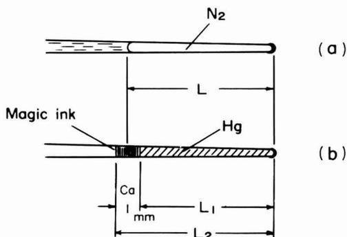
FIG. 3. Measurement of gaseous nitrogen by interpolation: (a) collected nitrogen, (b) nitrogen column has been replaced by a mercury column of roughly the same length.
