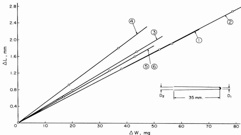
FIG. 4. Relationship between weight of mercury column and its length: ( $\Delta W$ ) differences in weight between shortest and longer mercury columns, ( $\Delta L$ ) differences in length between shortest and longer mercury columns, (1)  $d_1 = 0.25$  mm, (2)  $d_2 = 0.08$  mm, (3)  $d_3 = 0.32$  mm ( $D_2 < D_1$ ), (4)  $d_4 = 0.08$  mm, (5)  $d_5 = 0.7$  mm, (6)  $d_6 = 0.01$  mm ( $D_2 < D_1$ ), where  $d$  is differences of internal diameter between  $D_2$  and  $D_1$ .
