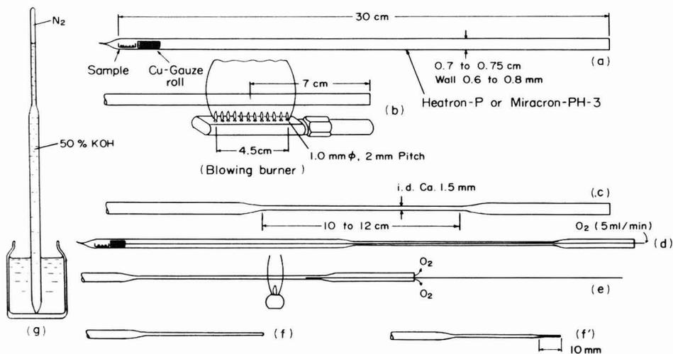
FIG. 1. Sweeping and sealing of combustion tube: (f) capillary for normal analysis, (f') capillary for measuring blank value.
