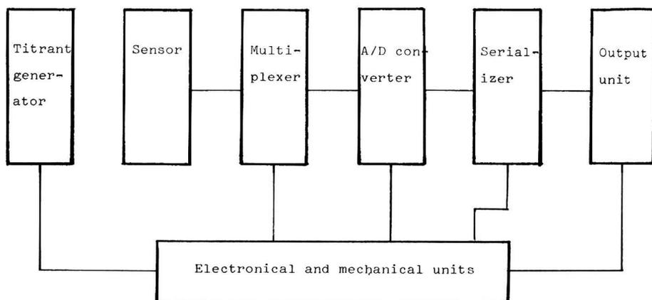
FIG. 1. Major parts of an off-line titrator.
