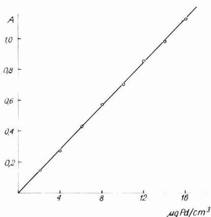
FIG. 4. The dependence of absorbance on palladium(II) concentration,  $\lambda = 540 \text{ nm}$ ,  $l = 1 \text{ cm}$ .
