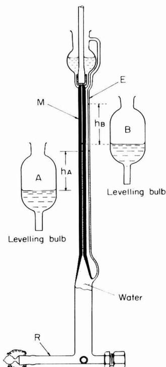
FIG. 3. Illustration of nitrometer: (A) level A, (B) level B, (M) calibrated measuring tube, (E) external parallel tube, (R) receiving chamber.
