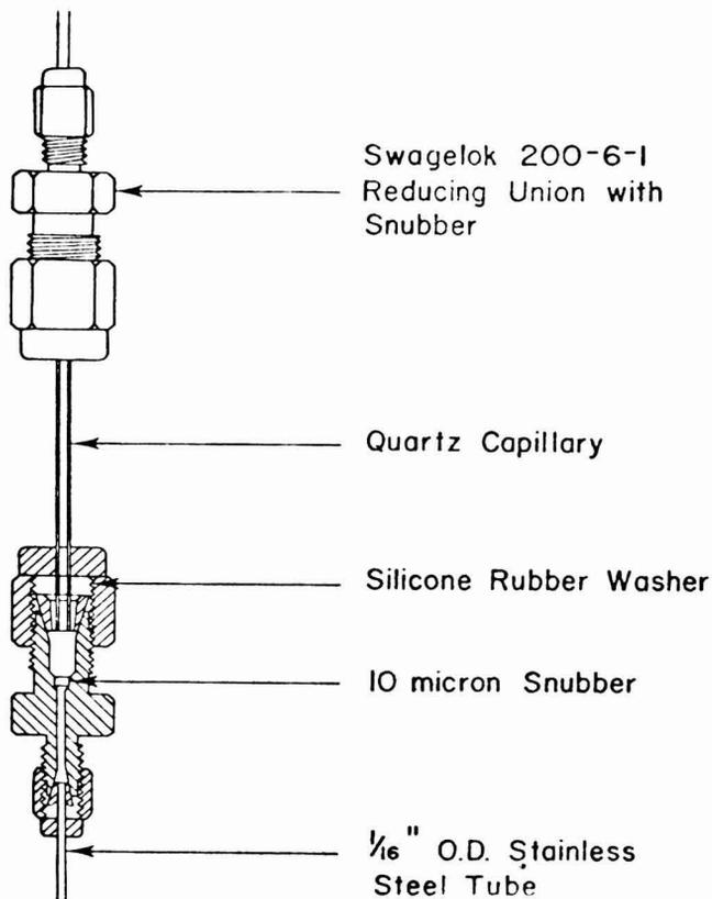
FIG. 1. Fluorometric flow cell.
