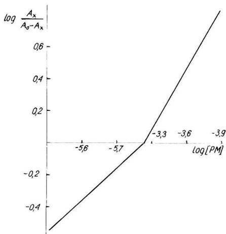
FIG. 3. The dependence's curve  $\log [A_x / (A_0 - A_x)]$  on promazine hydrochloride concentration, where  $A_0$ -absorbance of the solution after complexation all palladium(II),  $A_x$  increasing absorbance before complete complexation palladium(II) ions.  $C_{\text{Pd}} = 1.5 \times 10^{-4} M$ , acetate buffer of  $\text{pH} \approx 2.0$ .
