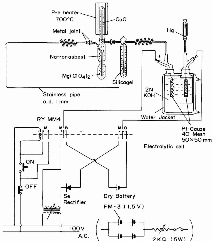
FIG. 2. Apparatus for supplying electrolytic oxygen: (RY) relay, (M) make conjunction, (B) break conjunction.
