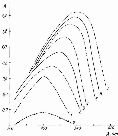
FIG. 1. Absorption curves performed in the system Pd(II)-PM at different molar ratio of Pd(II):PM, (where PM stands for promazine hydrochloride).  $C_{\text{Pd}} = 2.0 \times 10^{-4}$  M. (1) Pd:PM = 1:1; (2) Pd:PM = 1:4; (3) Pd:PM = 1:10; (4) Pd:PM = 1:20; (5) Pd:PM = 1:40; (6) Pd:PM = 1:55; (7) Pd:PM = 1:60. Acetate buffer of pH  $\approx$  2.0, (8) PdCl<sub>2</sub>,  $C = 1 \times 10^{-3}$  M.
