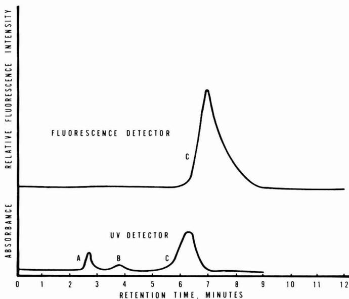
FIG. 4. HPLC chromatogram of 1,2-dichloroethane extract of pH 1.0 aqueous 50 ppb NO<sub>2</sub><sup>-</sup> sample. A. Excess DAN; B. sample matrix; C. triazole.
