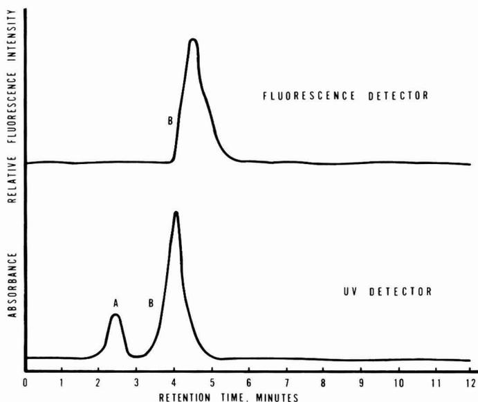
FIG. 5. HPLC chromatogram of chloroform extract of pH 1.0 aqueous 50 ppb Se(IV) sample. A. Septum bleed; B. DANSe.
