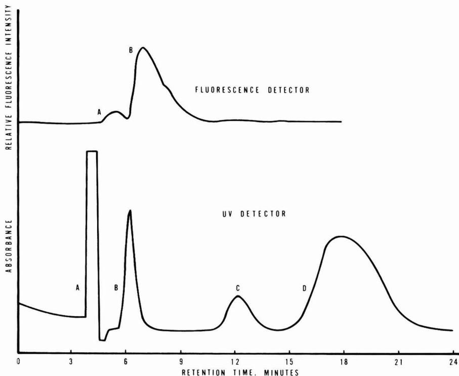
FIG. 2. HPLC chromatogram of pH 1.0 aqueous sample. A. Sample matrix; B. Triazole (1 mg/liter); C. DANSe (3 mg/liter); D. Excess DAN.
