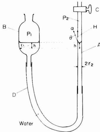
FIG. 1. Illustration of levelling operation: (A) graduated stem of nitrometer, (B) levelling bulb, (C) stopcock, (D) rubber tubing.
