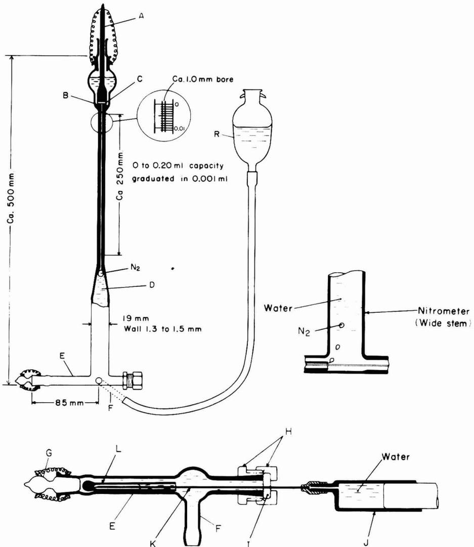
FIG. 1. Illustration of apparatus. A, plunger; B, nozzle; C, rubber sleeve; D, water; E, receiving chamber; F, side arm (connected with Tygon tubing to reservoir R); G, stopper; H, stuffing-box joint; I, rubber cap; J, hypodermic syringe; K, injection needle; L, capillary tube (containing nitrogen collected above KOH solution).
