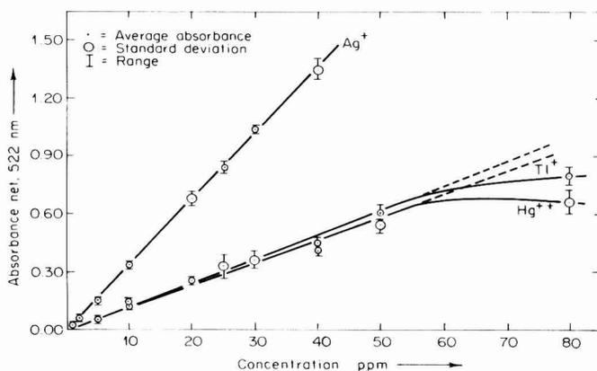
FIG. 1. Spectrophotometric response of the solid reagent as a function of  $Ag(I)$ ,  $Tl(I)$ , and  $Hg(II)$  concentrations.
