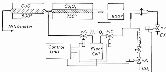
FIG. 1. Diagram of set-up.
