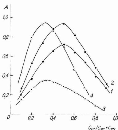
FIG. 2. Job's curves for isomolar solutions of PdCl<sub>2</sub> and PM. (1)  $\Sigma C = 1 \times 10^{-3}$  *M*, (2)  $\Sigma C = 1.2 \times 10^{-3}$  *M*. Acetate buffer of pH  $\approx$  2.0,  $\lambda = 460$  nm. (3)  $\Sigma C = 5 \times 10^{-4}$  *M*, (4)  $\Sigma C = 7 \times 10^{-4}$  *M*,  $C_{\text{H}_2\text{SO}_4} = 2.5$  *N*,  $\lambda = 540$  nm. Absorbance was measured at once after added solution of promazine.
