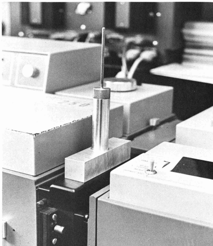
FIG. 1. Gilford Model 250 spectrophotometer fitted with rapid add/mix apparatus.
