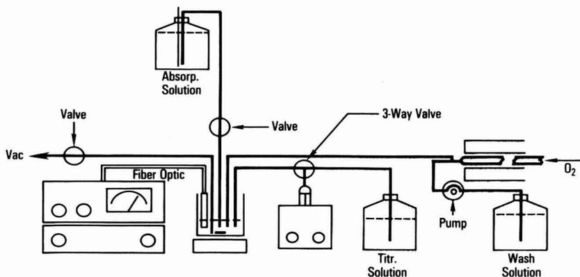
FIG. 3. Set-up for automatic sulfur determination.
