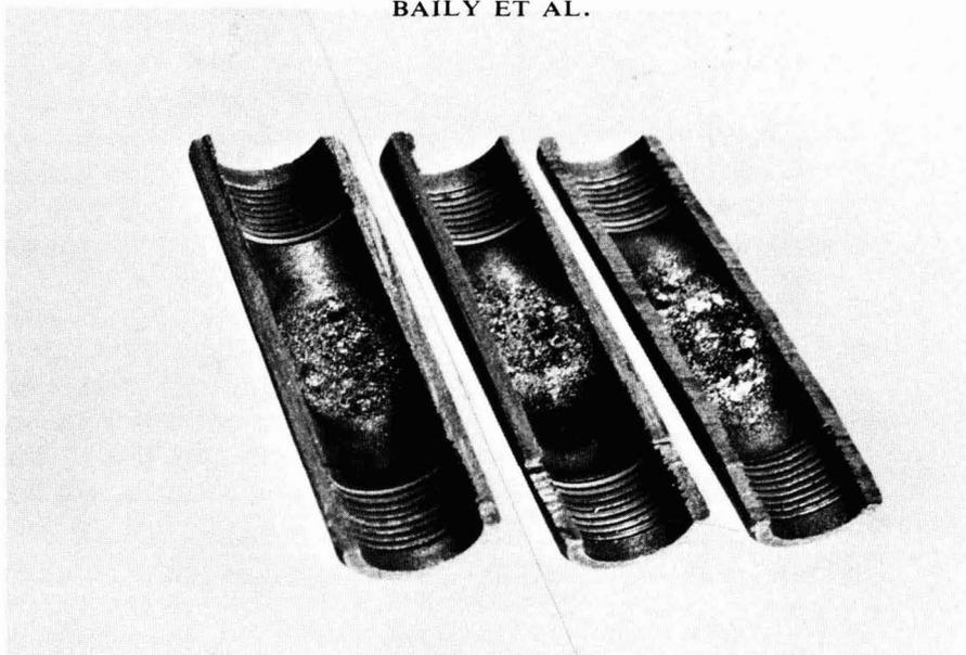
FIG. 3. Longitudinal section of untreated graphite tubes after approximately 200 firings showing residues from blood lead determinations.
