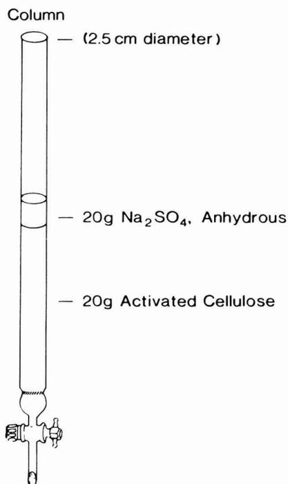
FIG. 1. Diagram of cellulose column.
