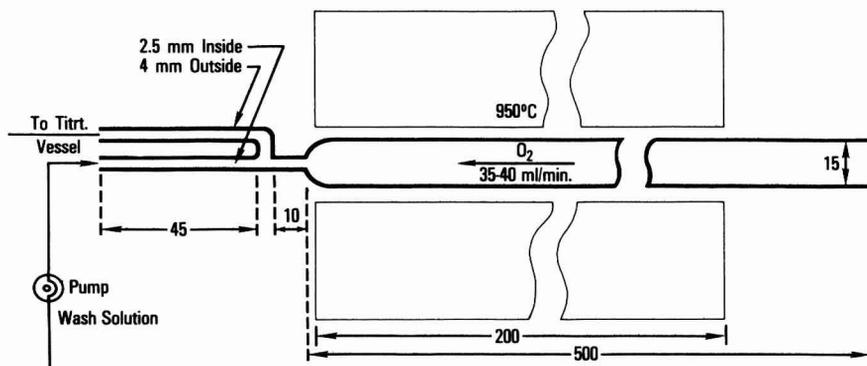
FIG. 1. Combustion tube with wash arrangement.
