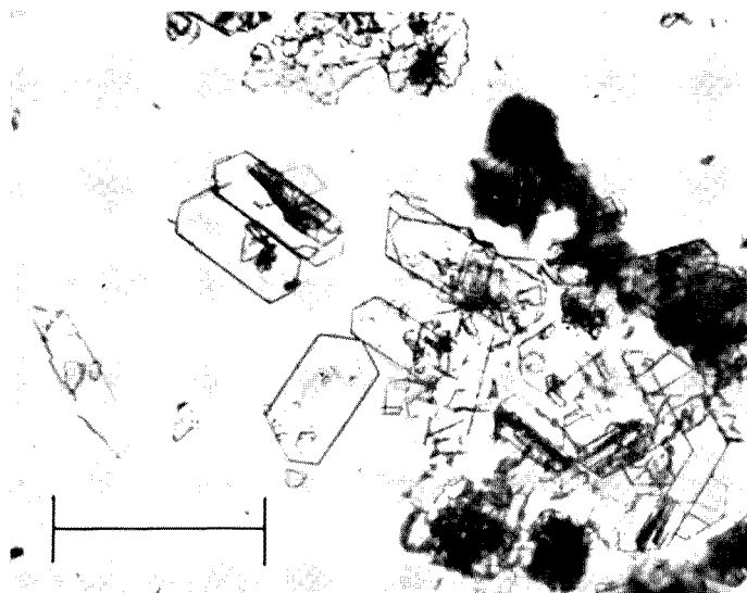
FIG. 2.—Nickel 8-hydroxyquinolate produced by solvent evaporation. (Distance shown is 0.1 mm.)
