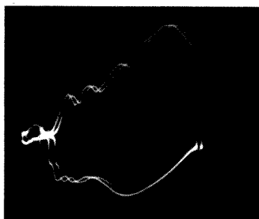
FIG. 12—Reaching equivalence in the determination of a mixture of dihydric phenols (electrolyte: 1M KNO_3 ; total phenol concentration: 6 \times 10^{-2} mg/ml; catechol:hydroquinone:resorcinol = 3:7:1; AC = 0.2 mA, DC = 2.0 mA).
