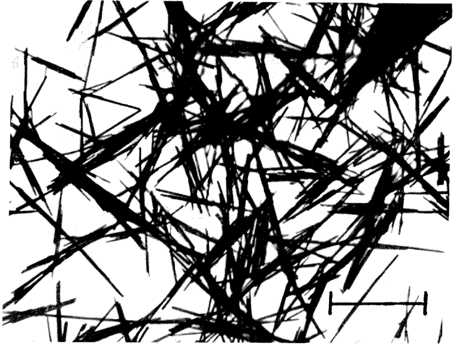
FIG. 3.—Nickel dimethylglyoximate precipitated by in situ generation of reagent (Distance shown is 0.1 mm in all Figures)
