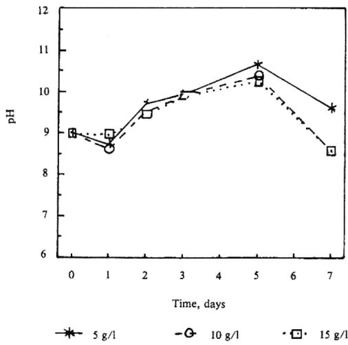
Figure 7 Changes of pH during growth of Spirulina SpT in outdoor at different concentrations of  $\text{NaHCO}_3$
