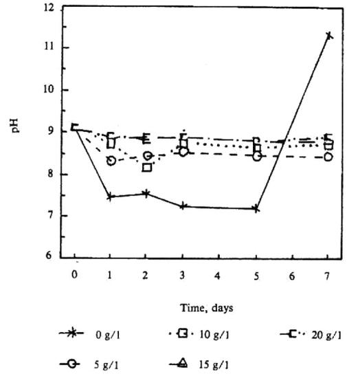
Figure 4 Changes of pH during growth of Spirulina SpJ in indoor culture at different concentrations of  $\text{NaHCO}_3$
